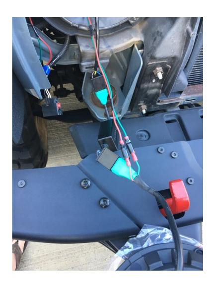
8. The main headlight wiring connector to light connector may not properly secure/clip in – if you are unable to get the clip to properly clip in and secure, you may opt to ensure the connection is secure and use a zip tie as shown
