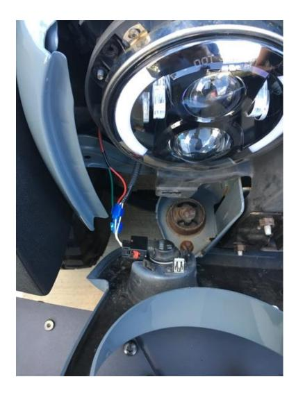
11. Complete the installation of the grille and when installing the push pins to secure the grille, make sure to orient the push pins as shown so it is easier to remove them in the future with a flat head screw driver.
