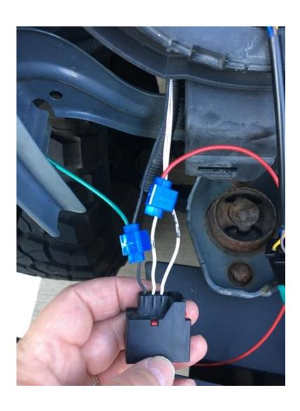
5. The original wire harness with the plug for the headlights will have two bare wires (red and green) protruding from the harness at the first wiring harness adapter to the light. These two wires are for the partial halo's and need to be connected to the day time running lights (DRL)/amber blinker below each headlight otherwise they will not illuminate when you turn on the lights (optionally they could be connected to the fog lights in the bumper using a similar procedure).
