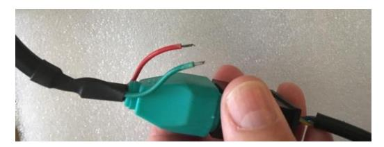
6. Strip off more of the wire sheathing so there is at least 3/8" wire exposed and install one half of the bullet connector to each wire (shown is the female connection). Do this for all four wires.
