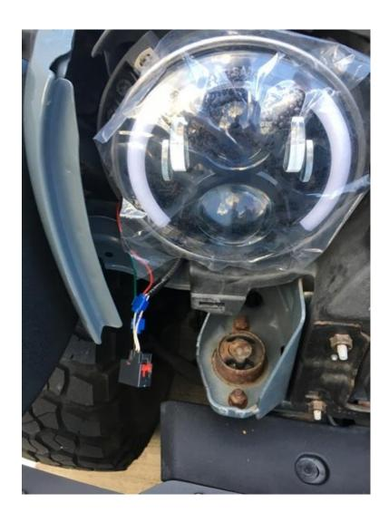
10. Before installing the grille complete, hook up the amber blinker connection to the light on each side and power up to make sure everything works before closing everything in.
