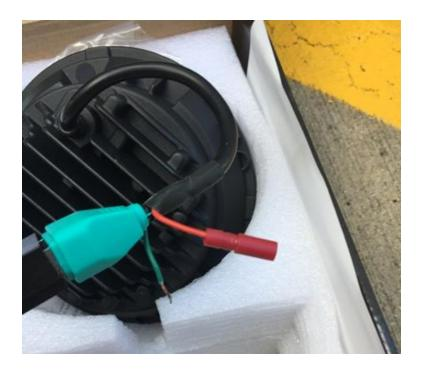
7. Once all the female ends of the bullet connectors are installed on the light harness, it is time to install the lights and make the wiring connections at the bullet connectors – make sure to connect the green to green and red to red. Not installed yet is the connection to the amber blinker which is still installed in the grille (only the wiring harness was disconnected on removal).
