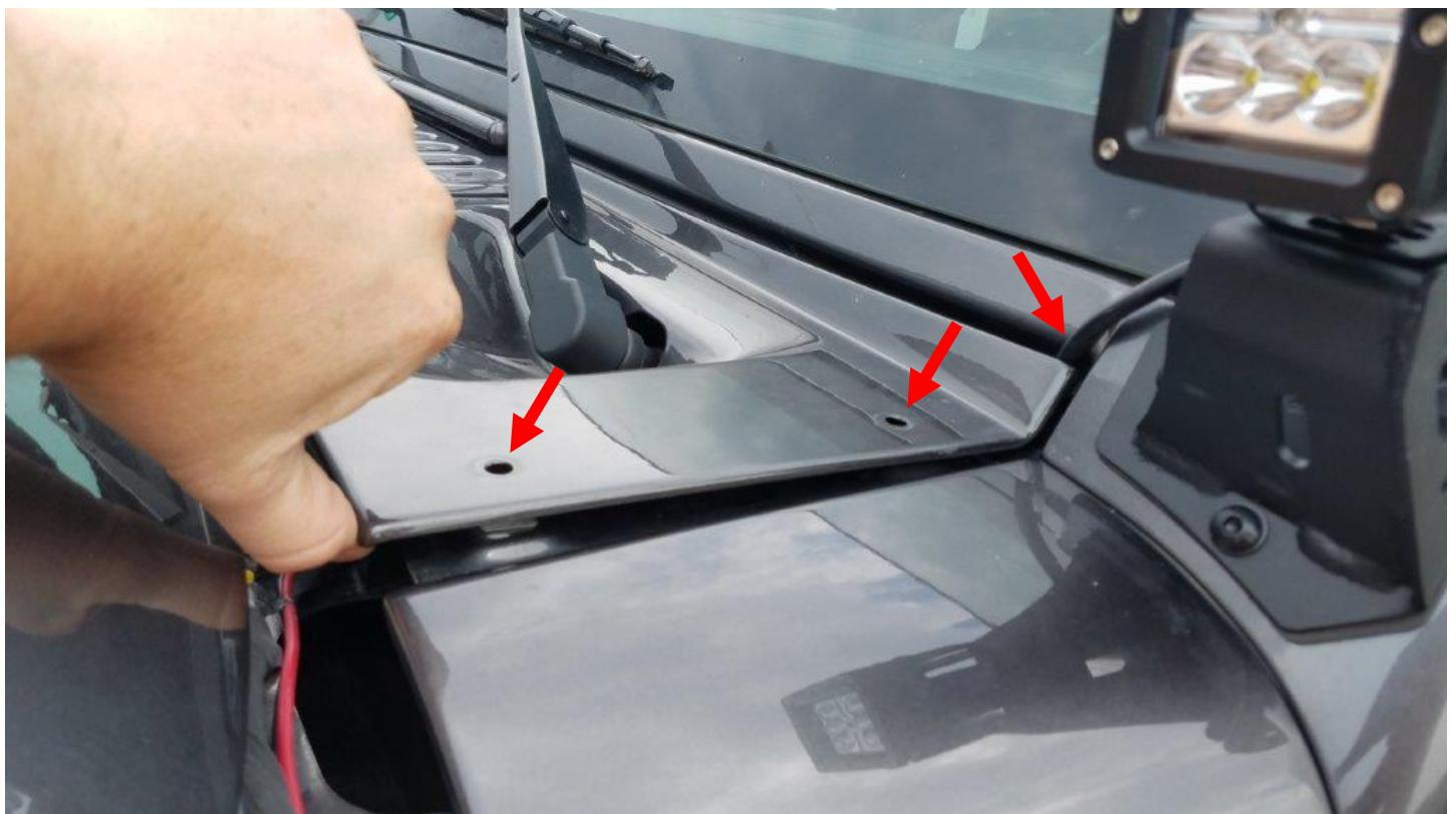
9. Route the wires to your power supply. I am using the Rough Country MLC-6, but it will be similar for most switching pods on the market. Make sure you keep the wires away from moving parts, and hot parts to keep them safe. Use zip ties to keep them in place.
