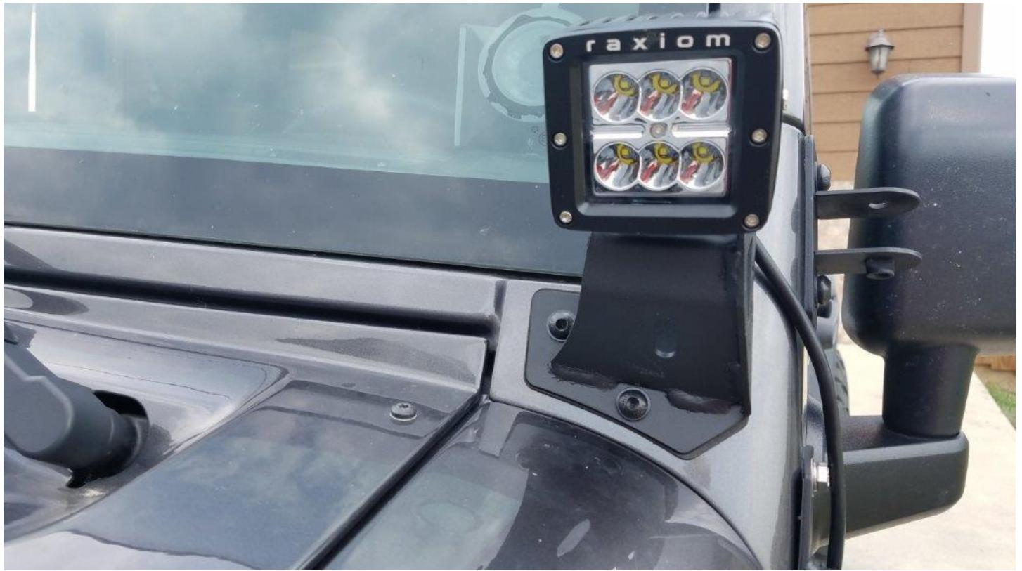
8. Open your hood. Use your T25 bit to remove the 2 screws holding this panel down. Then route the wire under the panel and into the engine compartment. Do this for each light on both sides of the Jeep. Then reinstall the T25 bolts.
