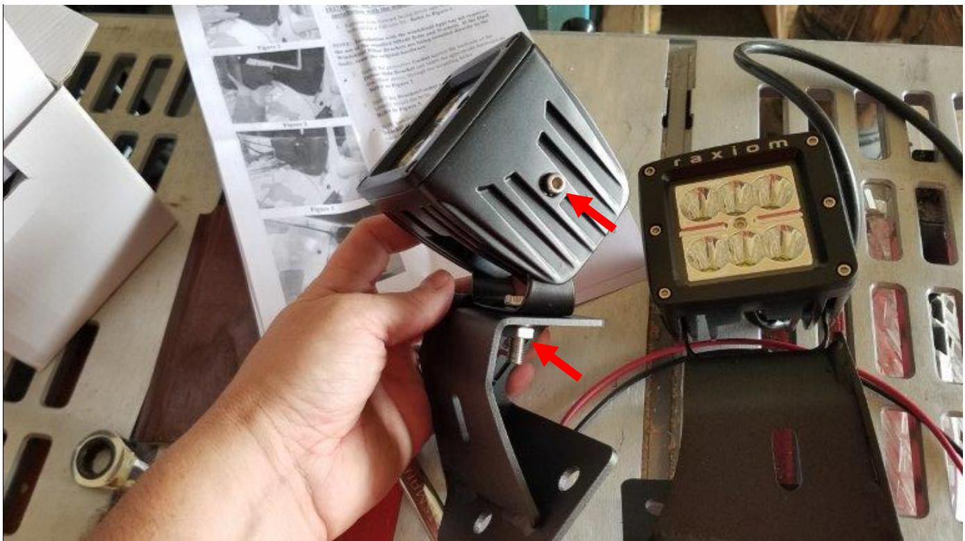
7. Then mount both brackets using your bracket specific mounting instructions. Adjust the aim of the lights as you desire, and tighten all hardware from step 6.
