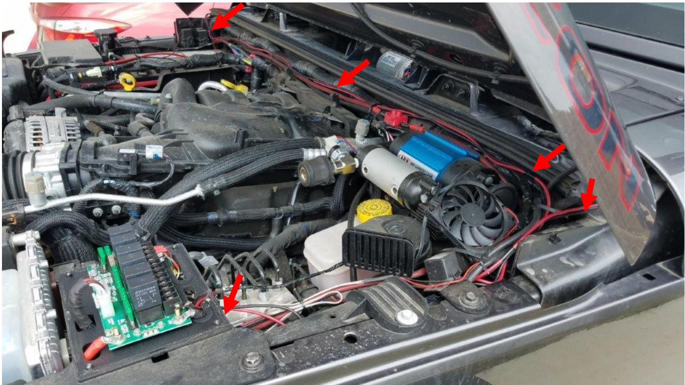
10. Attach the both red to the positive and the both black to the negative terminals on your switch pod.
