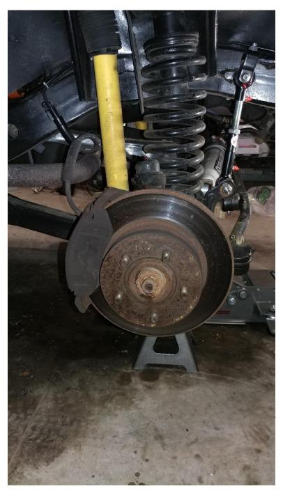
2. To remove the rotor the caliper must be removed first. Remove the 2-12mm bolts holding the caliper on.
