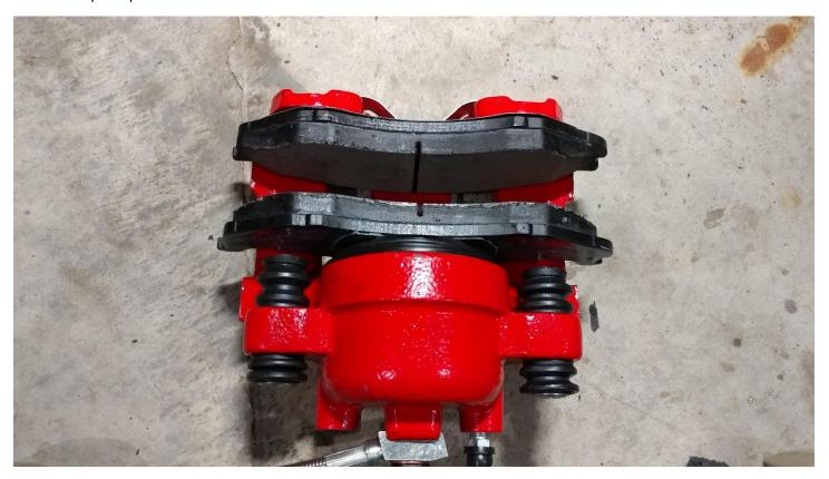
10. Starting with the top of the caliper insert the caliper and push down on the lower side.
