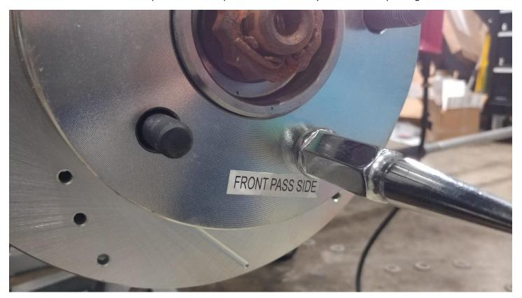
7. Use a lug nut to hold the rotor in place.
