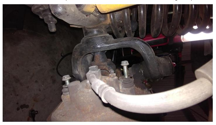
3. Lift from the bottom of the caliper to remove the caliper from the mounting position
