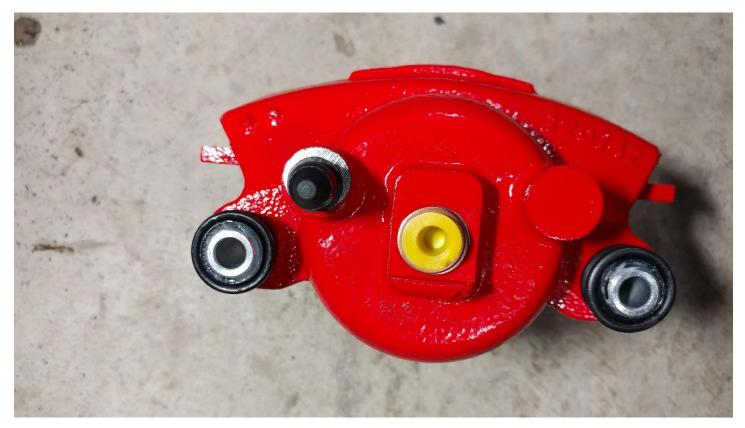
7. Use the 14 mm bolt to attach the brake line to the new caliper
