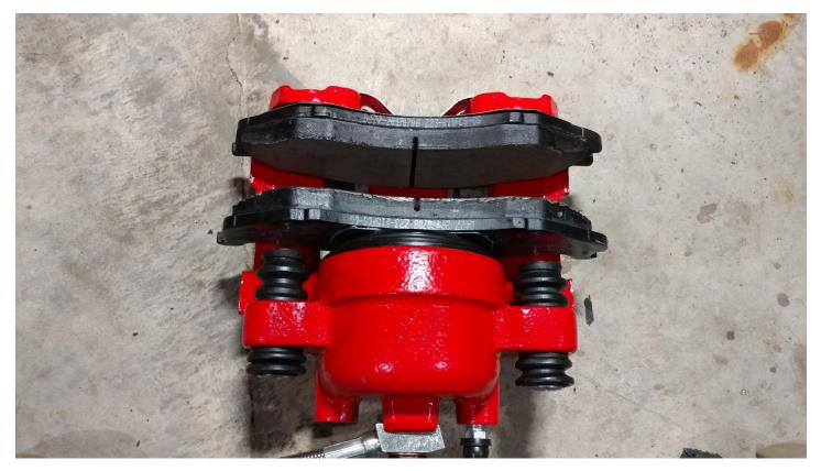
12. Reinstall the caliper using the new provided 12 mm bolts
