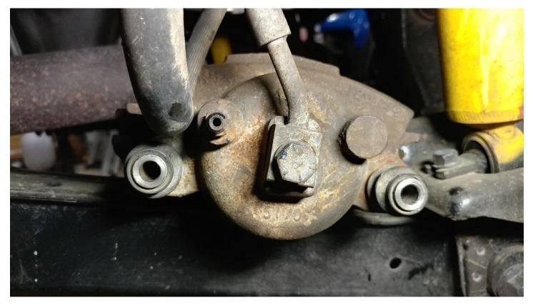
5. The brake fluid with leak until installed into the new caliper. Watch the fill reservoir to make sure it doesn't get low.
