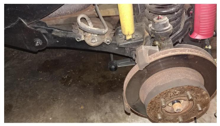
4. Using a 14 mm socket remove the brake line from the old caliper
