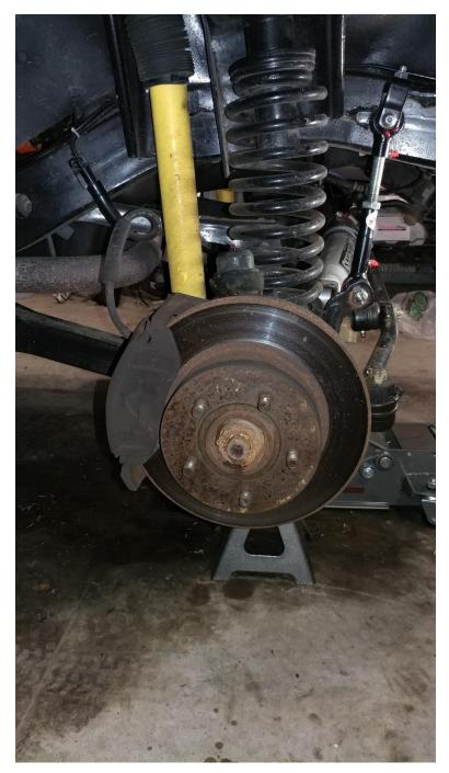
2. Remove the 2 – 12mm bolts holding the caliper on.
