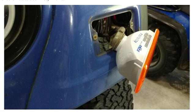
6. When reinstalling the new Omix-ADA Turn Signal Parking Lamp Assembly line up the pins located on the Omix-ADA Turn Signal Parking Lamp Assembly with the cut outs in the fender.
