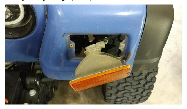
4. While grabbing the Turn Signal Parking Lamp Assembly with one hand and the light socket with another rotate counter clock wise, 1 half turn.
