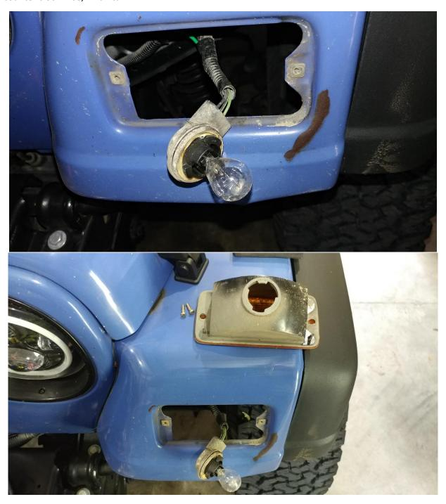
5. While grabbing the new Omix-ADA Turn Signal Parking Lamp Assembly with one hand and the light socket with another rotate clock wise, 1 half turn.
