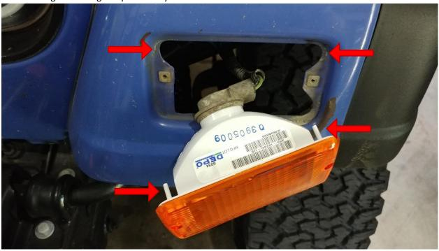
7. Reinstall the 2 factory T10 star screws, installation complete
