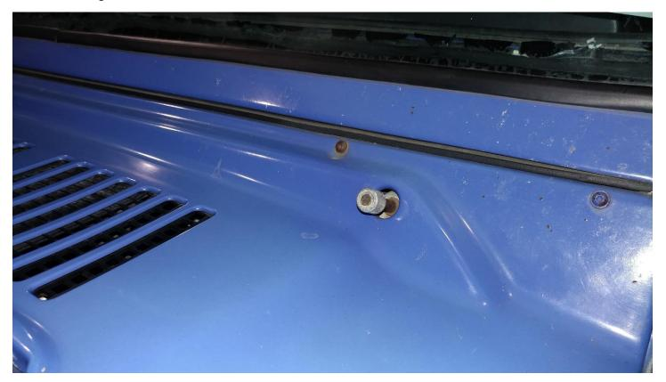
5. Using a flat head screw driver push down on the tabs shown
