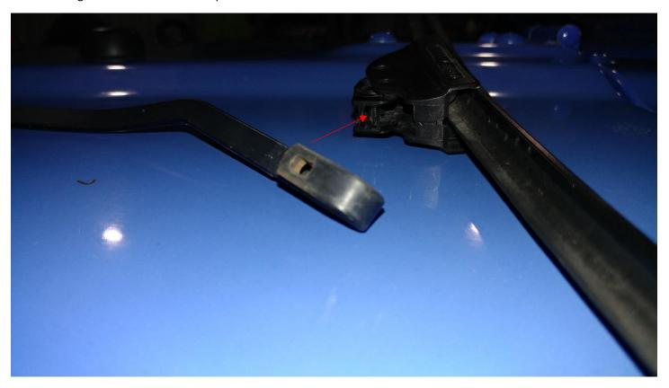
6. Attach the new wiper arm to the wiper blade assembly
