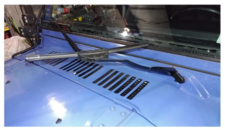
3. Pull the tab down from the lower side of the wiper arm where it attaches to the Jeep
