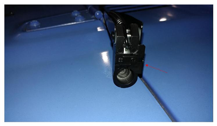
10. The wiper arm may have to be pushed on and pull off multiple times so that the correct position can be found. The wiper arm should slide on to the splines with minimal force.
