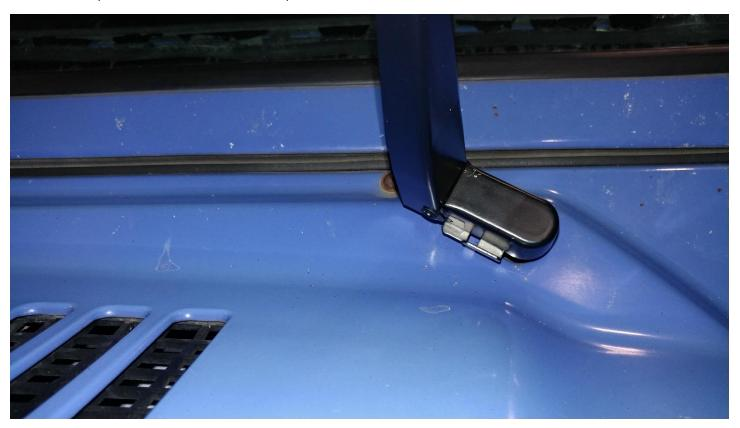
11. Once the proper angle is found push the tap up while the arm is bent
