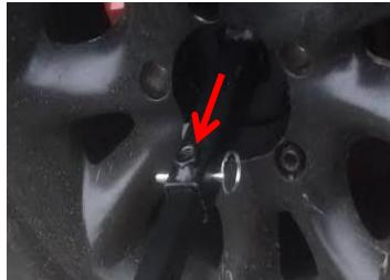
5. Place basket over cargo extension support bar and line up the hole with the preferred mounting point on the extension bar as it is adjustable. Place 1/4" Pull Pin through hole.
