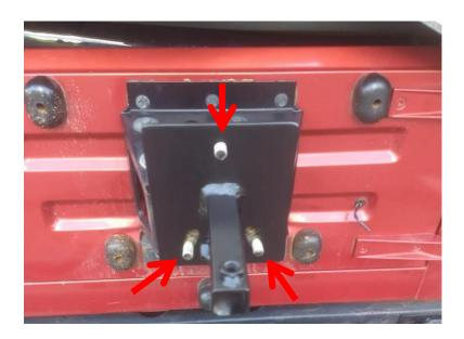
**3.** Remount spare tire over mounting bracket and tighten lugs between 40-80 FT-Lbs with a Torque Wrench or tight enough the tire is secure.
