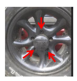
2. With the spare tire removed, place the mounting bracket over the spare mounting threads. If the two mounting bolts are at the top and one on the bottom, flip the plate upside down as it's universal for aftermarket mounting applications.
