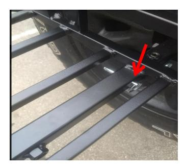
**6.** Place the other 1/2" set screw in the cargo basket and hand tighten with the Allen Wrench. Again do not overtighten as you could strip it.
