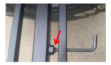
**7.** Your installation is now complete. To remove cargo basket, simply remove pull pins and set screws.
