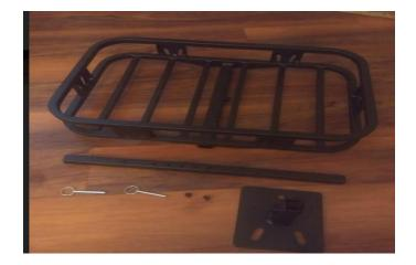
\*\*\* You will reuse your 3 spare tire mounting bolts for the mounting plate. This item can be used without the \*\*\* spare tire mounted, but may require shorter bolts.
