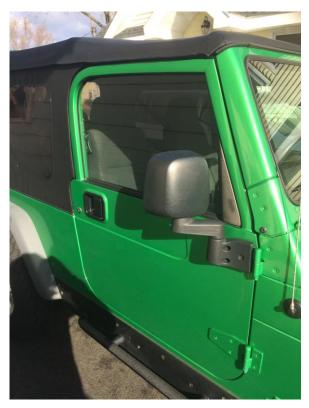
Before instillation both doors will need to be removed if they have not been already. Removal varies slightly by model. On this 2005 model the doors are removed by removing the two 13 mm nuts on the bottom of the door hinges. Once the nuts are removed the doors can be lifted off. Take care in removing doors as they are heavy. If installing safari doors consult the directions and install doors before installing mirrors.
