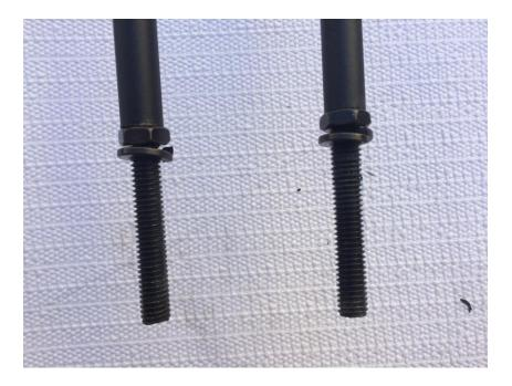
4. Slide the threaded rod of the mirror arm into the upper door-mounting bracket or mirror-mounting bracket on safari door.
