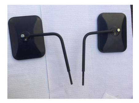
3. Install 1 jam nut (short) and 1 lock washer on the threaded rod of the mirror arm. Tighten with the 9/16-inch wrench.
