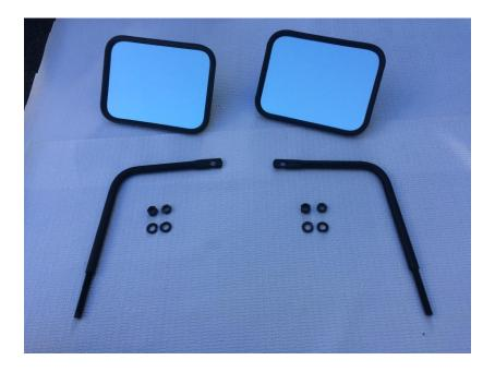
Attach the mounting arms to mirrors. Remove the bolt on back of mirror using the 13 mm wrench. Insert the bolt through the hole in the mounting arm and back into the hole in the back of the mirror. Tighten securely. Repeat on other mirror making sure to reverse direction of the second mirror so when installed both mirrors will face to the rear of the Jeep.
