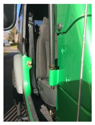
5. Install lock washer and nut onto threaded end of rod from bottom and tighten with the 9/16-inch wrench.
