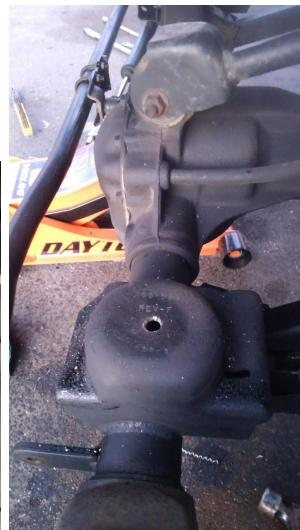
10: Once bump stops are installed, install the new Old Man Emu Front Springs!
