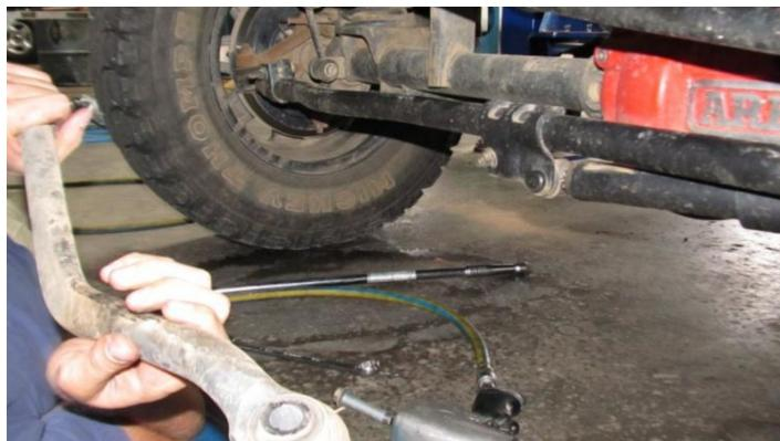
3: Lift vehicle and support with jack stands so you have enough room to drop the front axle.
