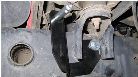
13: Fit the sway bar disconnect park brackets to the chassis rails. This may require a hole to be drilled on some models.
