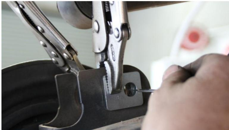
4: Using a die grinder, cut the marked area.
