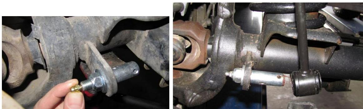
15: Fit brake line drop brackets using the fasteners provided.
