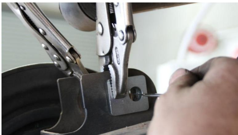
4: Using a die grider, cut the marked area.
