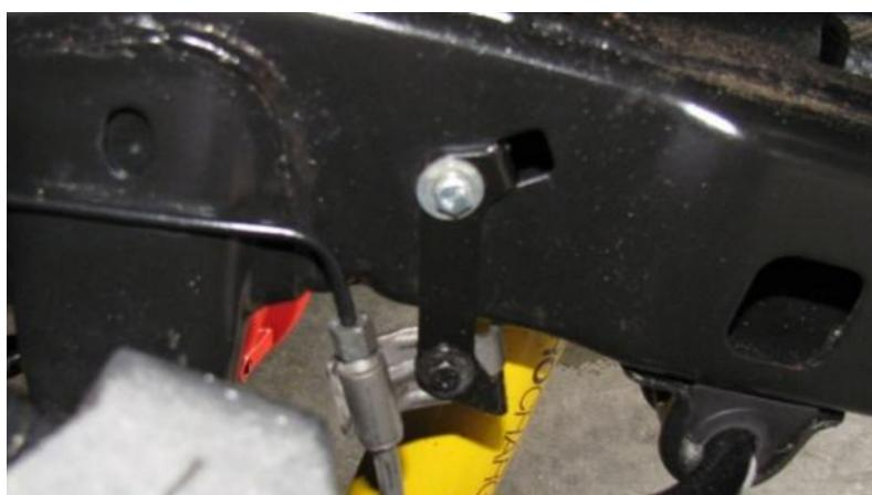
14: Fit the hand brake relocation bracket as shown.
