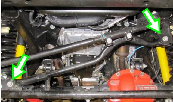
19: Once axle is centered, adjust drag link to re-centre the steering.
