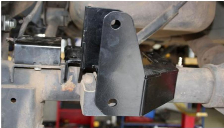
8: Clamp the track bar bracket in position with the 2 U-bolts provided.
