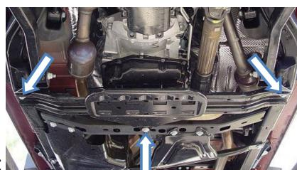
1: While at ride height, remove the top shock absorber mounting nut, washers and bushings using a 16mm wrench.
