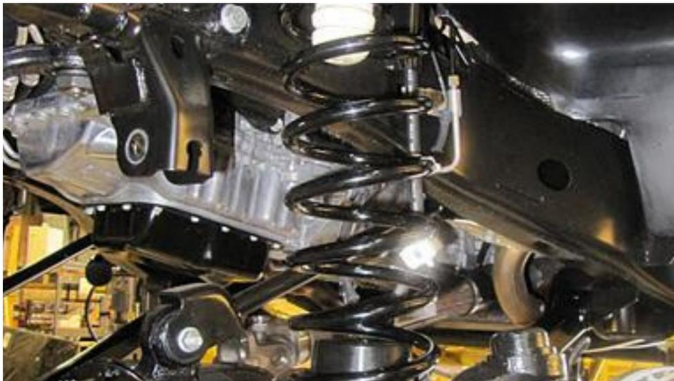
11: Fit the new BP-51 Shock Absorbers as per the instructions that come in the box. First mount the top of the shock, then raise the axles back up pinching the springs into position and lining the lower shock absorber holes up with the spots on the axle to mount them to.
