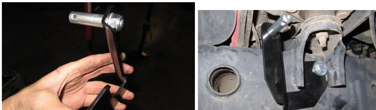
13: Fit the sway bar disconnect park brackets to the chassis rails. This may require a hole to be drilled on some models.
