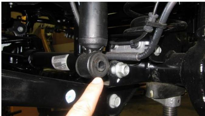
8: Lower the axle far enough to pull out old coil springs, but watch for brake lines and sensor wires to prevent breaking when lowering the axle. When its low enough, remove the springs.
