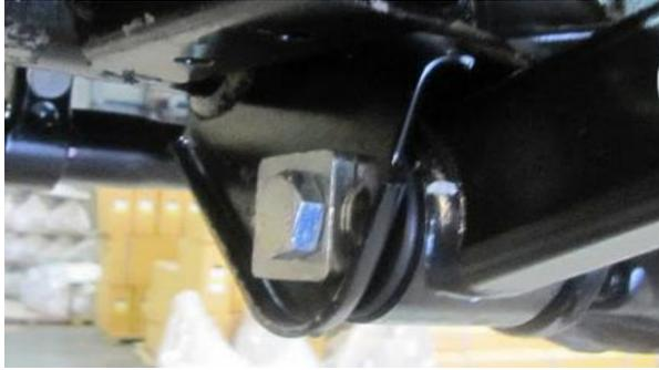
5: Reposition alignment plates and reconnect the lower control arms using the hardware supplied. Do Not torque at this stage.
