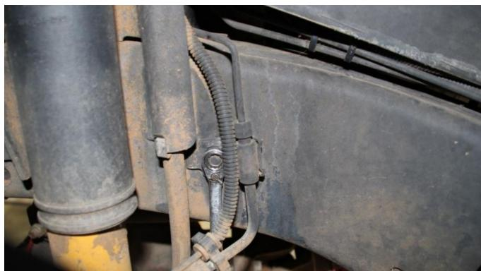
6: Remove front sway bar end links on both sides of the front sway bar.
