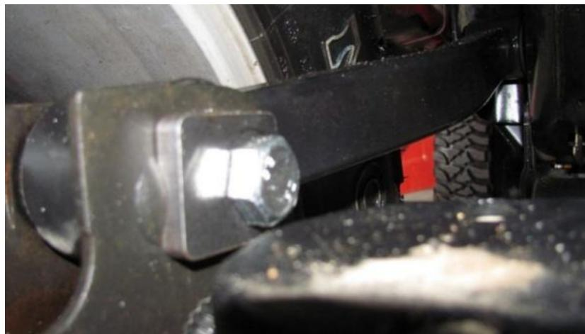
7: Fit the new rear track bar bracket to the rear axle as shown.
