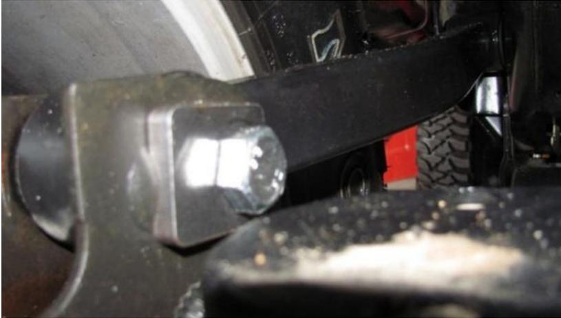
7: Fit the new rear track bar bracket to the rear axle as shown. Re-fit the original bolt and nut back in their original positions with the new spacer tube fitted in the original track bar position.
