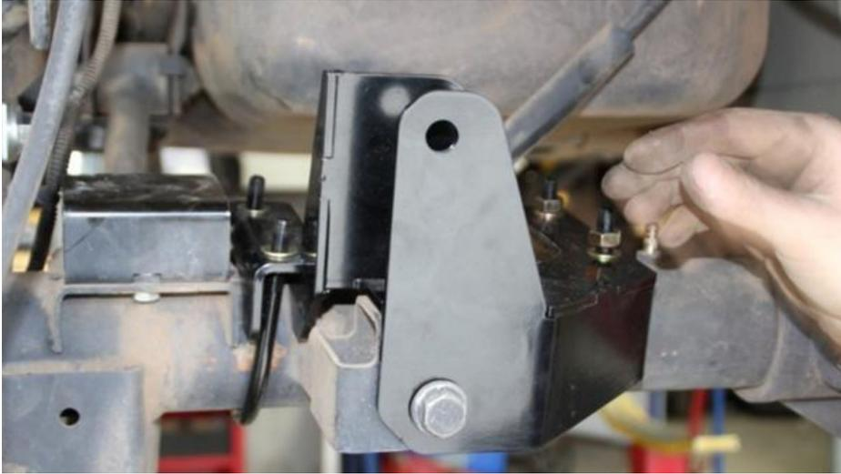
9: Fit the track bar to the new bracket using new bolt and nyloc nut and flat washers provided.
