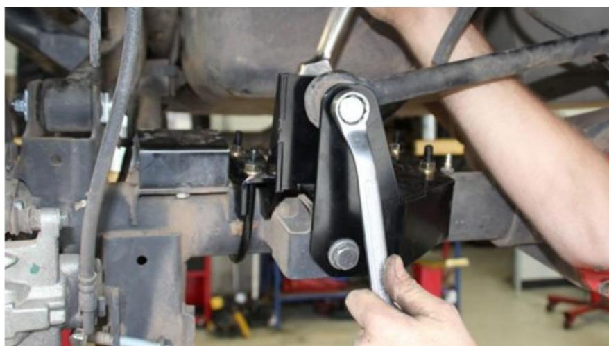
10: Fit the rear bump stops using the fitting instructions provided in the kit.
