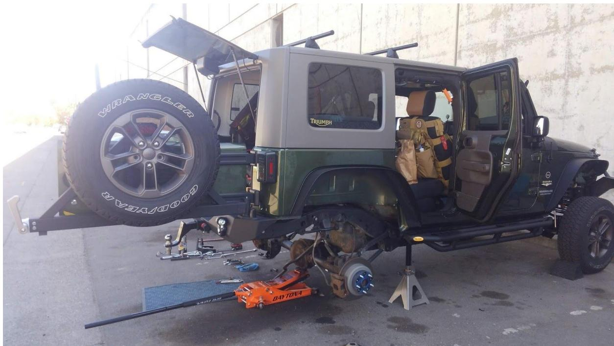
2: Disconnect brake line brackets on both sides.
