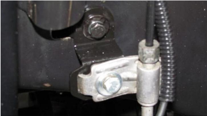
16: Make sure your front differential breather tube is relocated allowing t=for increased wheel travel. Use included zip tie.
