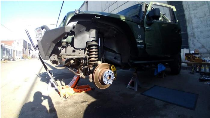
4: Remove front wheels and drop axle down a couple of inches after the frame rests on the stands. This will give you more room to avoid head bonking.
