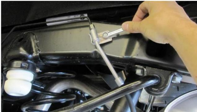
3: Remove rear sway bar links on both sides.
