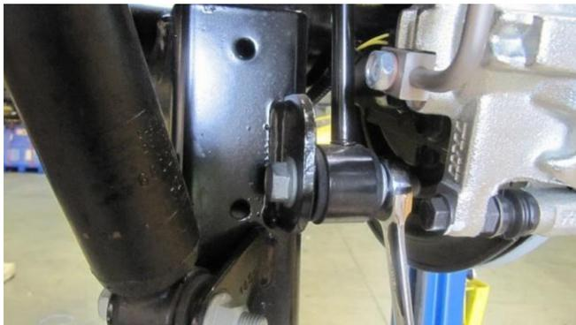
4: Disconnect rear track bar at the axle end and loosen chassis end.
