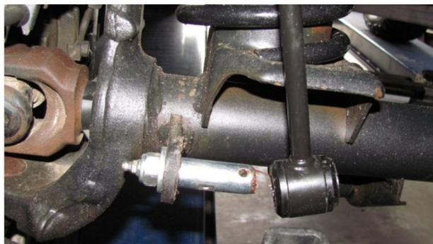
15: Fit brake line drop brackets using the fasteners provided.
