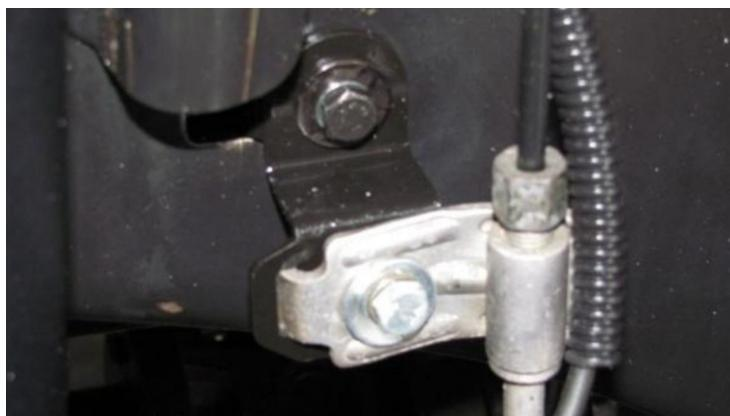
16: Make sure your front differential breather tube is relocated allowing for increased wheel travel. Use included zip tie.
