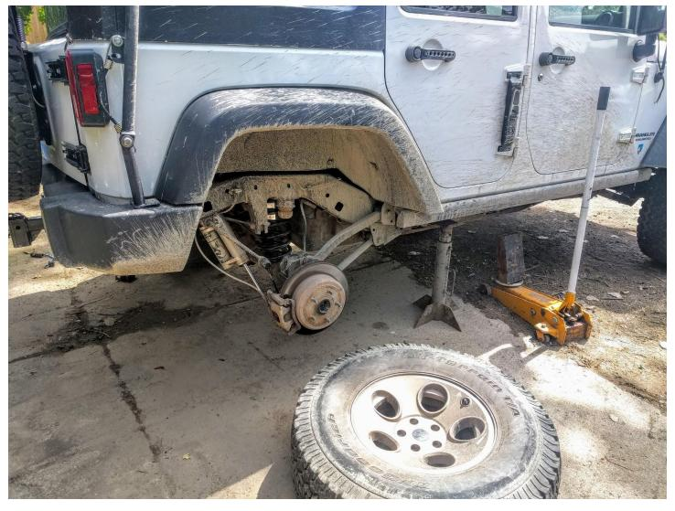
2. After verifying that tension is off of the sway bar link (adjust tension by raising the jack still under the axle), Use a pair of 18mm wrenches or ratchets to remove axle side of sway bar link. Lower axle as necessary and use same wrenches to remove lower bolt from shock.
