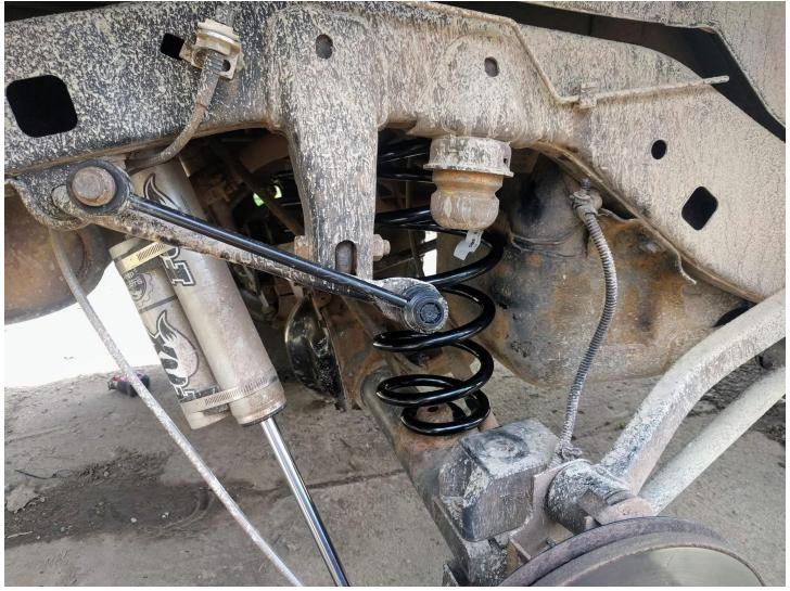
5. Rotate the spring on the lower perch until it settles into place, then use jack to raise axle and replace bolt through shock mount, (it is recommended to wait to torque shock bolt to spec after vehicle is resting at ride height and on all 4 wheels). Raise axle further and reconnect sway bar link. Now reconnect diff breather hose, brake line bracket, wire loom clips, etc that were loosened or removed during installation. Reinstall wheel and lower vehicle. Now torque lower shock bolt.
