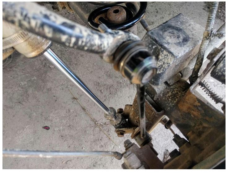
3. After verifying that all necessary brake line brackets and wire looms are loosened as needed, carefully lower axle. You will likely be able to simply remove existing spring by hand at this point. Or use a prybar for a little persuasion.
