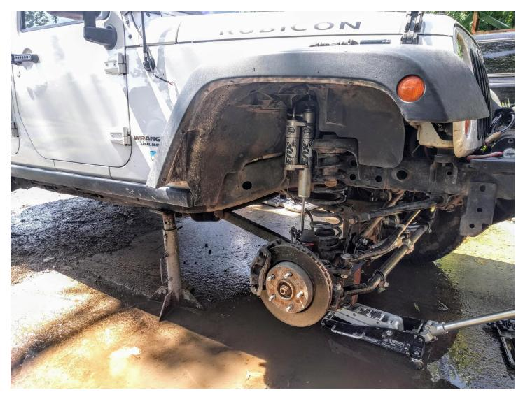
2. After verifying that tension is off of the sway bar link (adjust tension by raising the jack still under the axle), Use a pair of 18mm wrenches or ratchets to remove axle side of sway bar link. Lower axle as necessary and use same wrenches to remove lower bolt from shock (not pictured).
