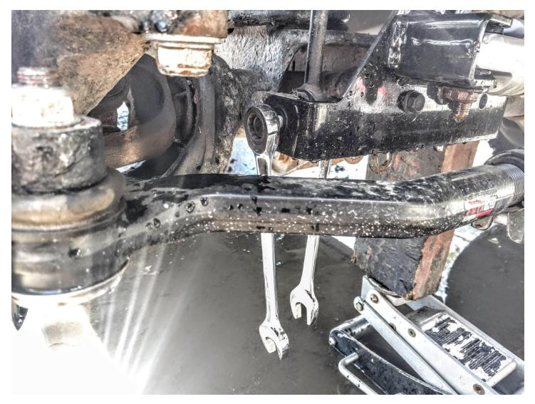
3. After verifying that all necessary brake line brackets and wire looms are loosened as needed, carefully lower axle. You will likely be able to simply remove existing spring by hand at this point.
