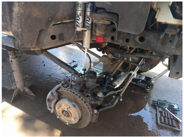
4. Reusing rubber upper spring isolater, slide new spring into place on upper tower, and then using your favorite method of axle manipulation/spring compression, slide new spring into place on lower perch. I typically use a 3ft prybar to lift spring into place from the bottom.
