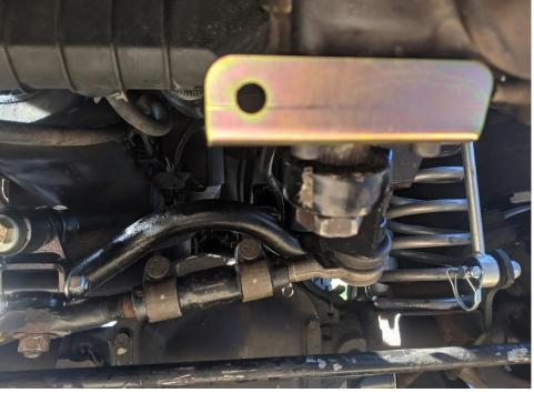
5. Push the 7/8" x 2-1/2" crush sleeve through the hole on the passenger's side of the frame; be very careful not to drop it into the frame rail. (If dropped inside, a reach magnet can help retrieve it) Place the flat washer on the 5/8" bolt and thread it from the outside of the frame through the crush sleeve.
