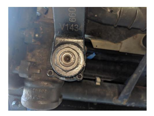
4. Once removed, slot the gold bracket on the steering box around the pitman arm and line up with the bolt holes. The bracket hole should face the passenger side of the vehicle. Apply a small drop of Loctite to the 8mmx1.25x35mm hex bolts. Install the 4 supplied 8mmx1.25x35mm hex bolts on the bracket into the stock threaded holes. Tighten these with the Hex Key Wrench until snug.
