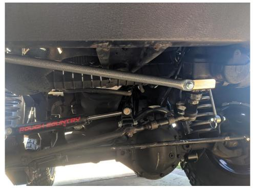
8. Congratulations! You have successfully installed the M.O.R.E. Powering Steering Box Brace on your 03-06 Jeep Wrangler. Recheck all the torque after 500 miles and following every oil change thereafter. This should not affect the alignment and center of your steering wheel. If it does, however, an alignment may be needed.
