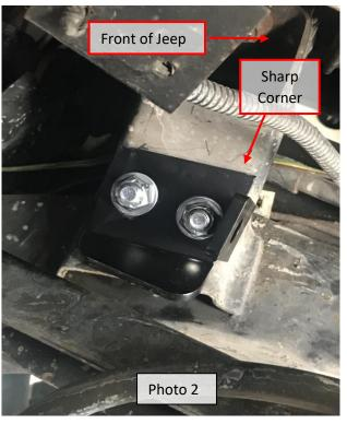
2. <u>J Brackets</u>: Set the J brackets next to each other on a hard surface. One of the brackets is longer. The longer bracket will be used on the driver's side. The flat face of the J brackets will face the front of the jeep. Attach the J bracket to the angle brackets you just mounted in Step 1 using 7/16" x 1-1/4" bolts, flat washers (on both sides of the bolt), and nuts. Leave the bolts loose at this time. See Photo 3.
