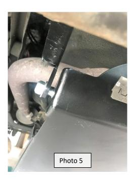
4. Align the skid plate so the large pre-cut hole is centered around the oil drain plug.
