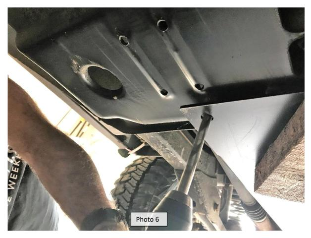
6. Making sure the TJOPSP is centered and you have clearance around the exhaust and driveline, tighten up all the nuts and bolts.
