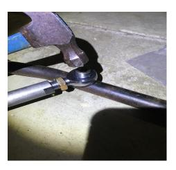
4. Adjust length of trac bar and tighten adjustment nuts with 7/8" wrench. Use longest bolt to mount the end of new trac bar with thicker bushings (shoulder spacers) on to back of frame mounting bracket.
