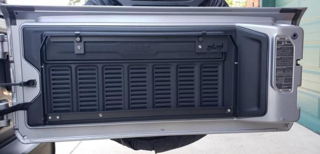
5. After securing the bracket to the tailgate it is time to attach the table. Place the table in the mount as if it were stowed away, hook the latches in place and secure those to hold the table in place while attaching the last pieces of supplied hardware. On both sides, slide the short T30 TORX screw from the outside, through the mount and table with Nylon spacer between the two and then hand thread the nut onto the screw.
