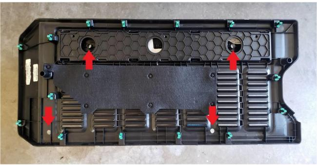
3. Now that the holes are drilled, attach the plastic trim back on the tailgate, ensure the trim in snapped back on securely by lightly tapping around the edges. Slide the provided Aluminum spacers into the holes that we just drilled, the longer Aluminum spacer should be inserted into the bottom left hole.
