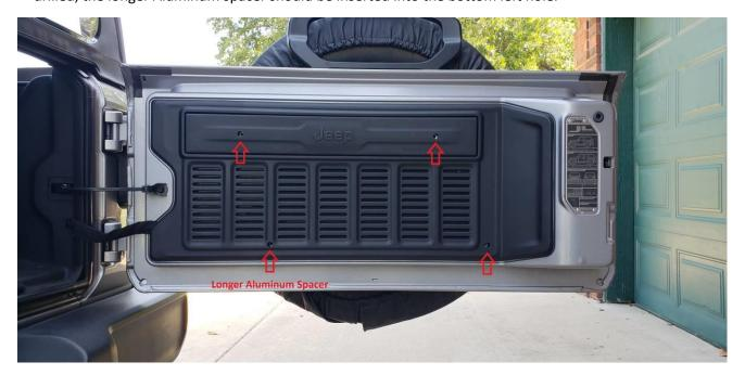
4. For the next step, mount the bracket beginning with the top two holes. Insert and hand-tighten two of the supplied long TORX screws with lock washers through the bracket and Aluminum spacers into the threaded holes on the tailgate. Before tightening the top two screws, insert and hand-tighten the bottom two TORX screws with lock washers through the bracket and spacers. Using a T30 TORX bit and ratchet or screwdriver, tighten down all screws.
