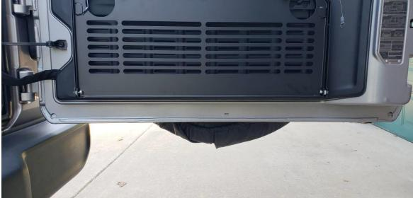
6. Once both sides are attached, use the 10mm box wrench to hold the nut in place while using a 3/8" ratchet and T30 TORX bit to tighten the each screw on both sides.
