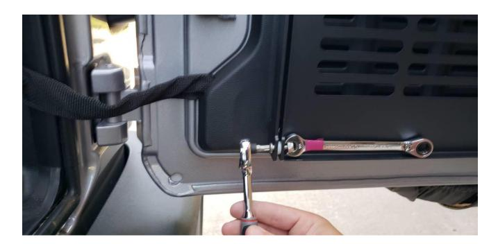
7. The final step is connecting the cables, lower the table down and the cables will simply loop over the stud on the inside of the mounted bracket.
