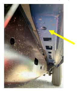
5. Now that your running board is held up by the hardware, tighten the (6) 10mm flange nuts and the (3) 13mm bolts. Please note, a 3" extension makes tightening the 13mm bolts easier.
