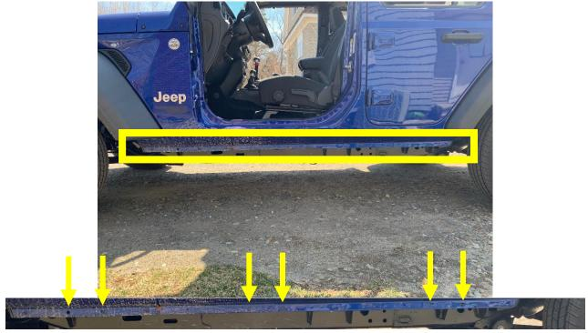
4. Locate the (3) threaded inserts on the bottom of your jeep and finger tighten (3) 13mm bolts.
