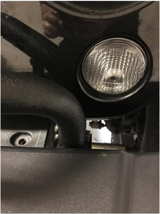
10. Fully tighten using included allen key wrench and 13mm socket and driver. Use care not to overtighten and flatten the light bar tube.
