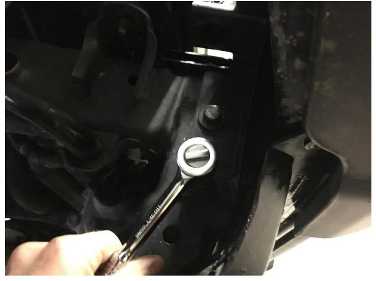
12. Reinstall the fasteners to the bumper frame cover and reinstall the front skid plate if previously removed. I like to use heavy duty zip ties for the skid plate since the fasteners have a tendency to wear out.
