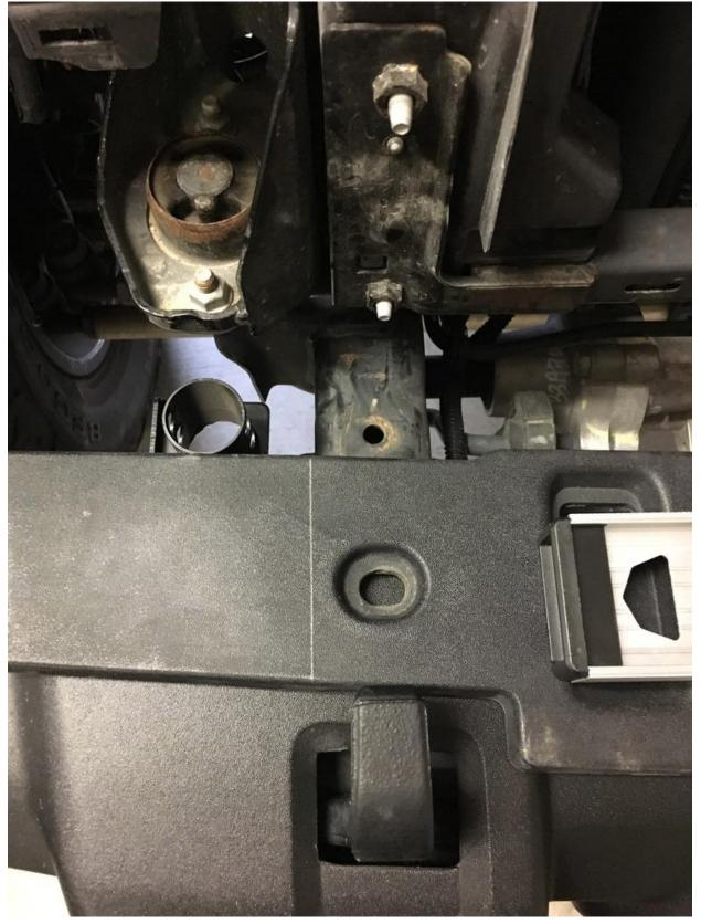
7. Slide the frame cover back into place, but do not yet install the fasteners in the event that the flange nuts need
