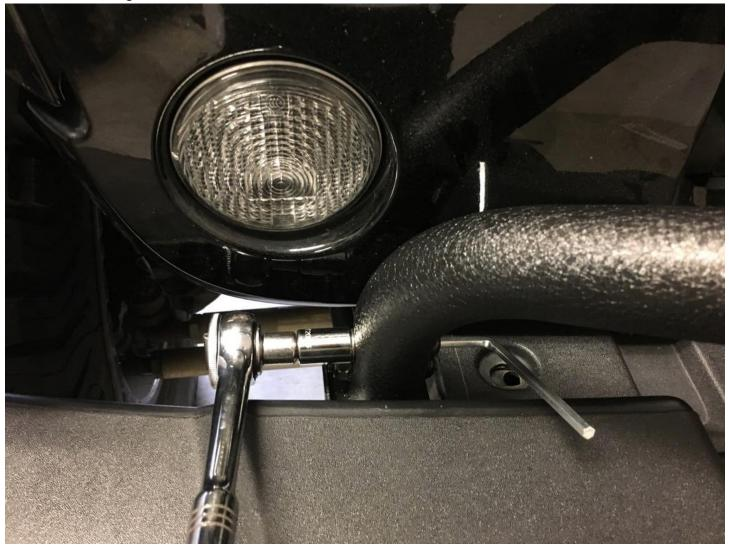
11. Using 18mm socket and driver, fully tighten the bolts securing the light bar mounting brackets to the bumper frame plate behind the bumper. Because the kit utilizes flange nuts, you should not need to provide backup to
