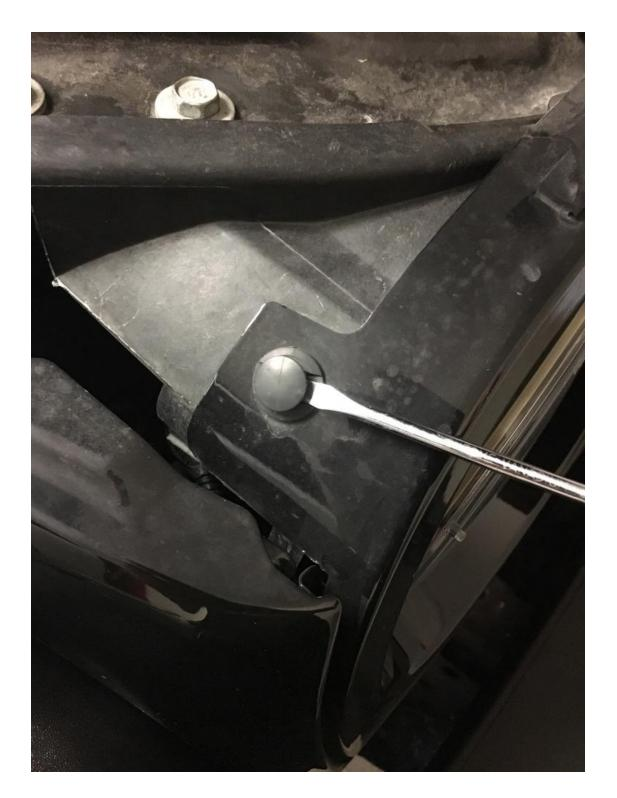
2. Using a phillips head screwdriver, remove the two fasteners from the front bumper frame cover, remove the cover, and set aside.
