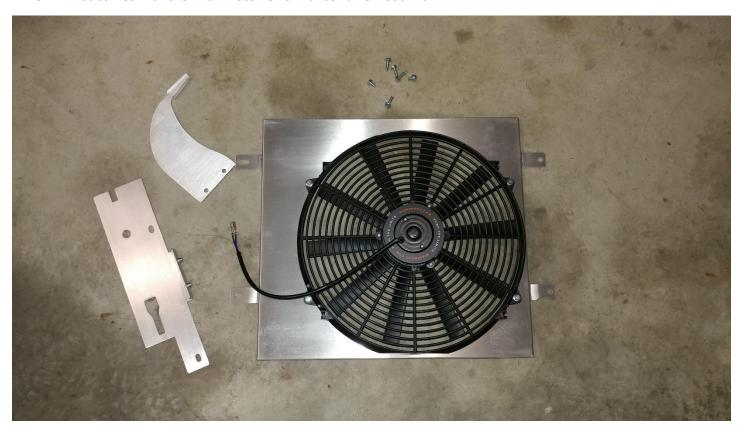
10. Install the fan shroud and overflow bottle bracket. The Mishimoto Performance Fan Shroud Kit did come with hardware but it did not work with my application. Reinstall the factory 8mm bolts.
