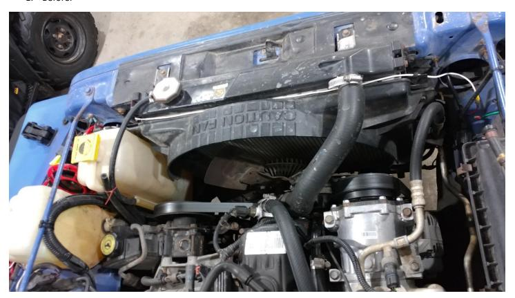
2. Remove the radiator overflow bottle. By pulling up from the bottom of the bottle.
