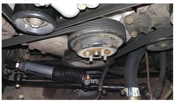
7. Reinstall the  $4 - \frac{1}{2}$ " nuts. This holds the water pump pully in place.
