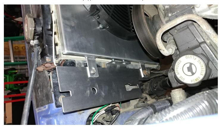
11. Reinstall the factory 8mm bolts on the passenger side.
