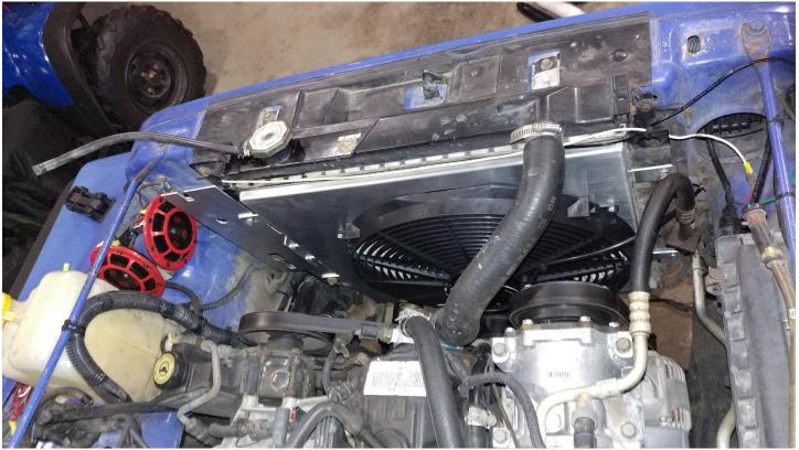
12. Reinstall the factory overflow bottle and connect the overflow line.
