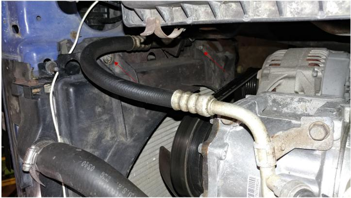
5. Remove the  $4 - \frac{1}{2}$ " nuts holding the fan on the water pump pully.
