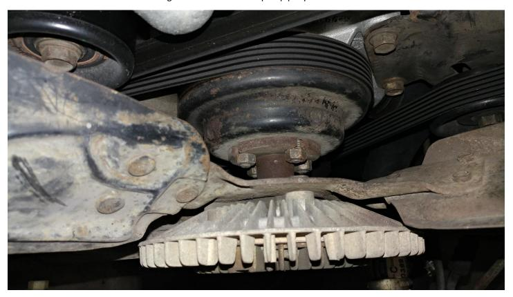
6. Carefully pull the shroud and fan from the Jeep. DO NOT HIT THE RADIATOR CORE.
