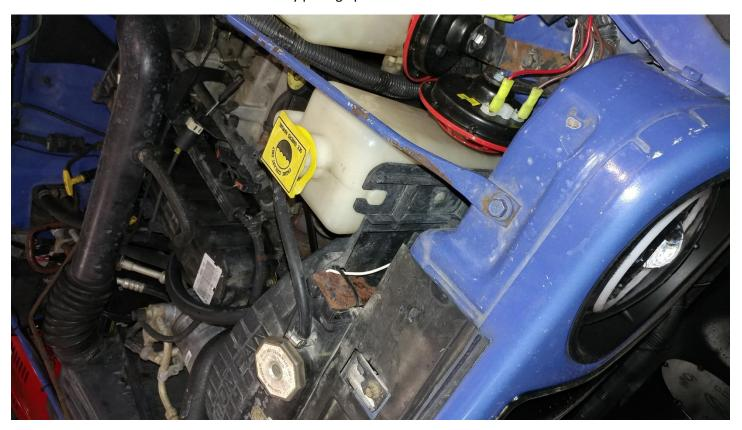
3. Disconnect the overflow line from the bottle using a pair of pliers.
