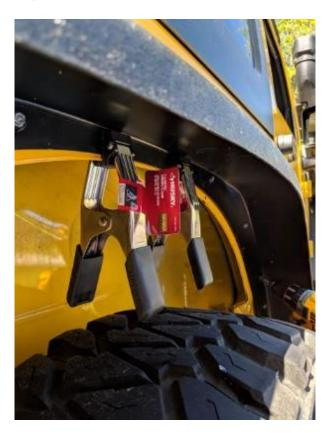
6. Once the fender is lined up, use the <u>drill with the 9/64"</u> to drill pilot holes. Then place the fender back in place and use the <u>drill with the 5/16" driver</u> to install the self-threading screws. Before drilling in each screw, coat it with a dab of <u>RTV</u> to help prevent rust. Do not tighten the screws initially.
