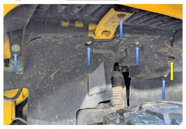
3. After you remove the bolts, the fender is still held on with several plastic clips. In order to remove the fender from the clips, grab the bottom of the fender on either side and pull up and out at the same time. It may take several tries and at first it will feel like it's not going to budge, but keep at it and it will pop off of the clips little by little.
