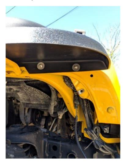
9. To fully secure the fender, use the <u>drill with the 5/16" driver</u> to install the self-threading screws. Before drilling in each screw, coat it with a dab of <u>RTV</u> to help prevent rust. Do not tighten the screws initially.
