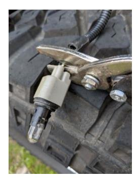
12. Using the <u>wire stripper</u>, strip about 1" off both the black and white wires from the Jeep and from the new corner marker lights.
