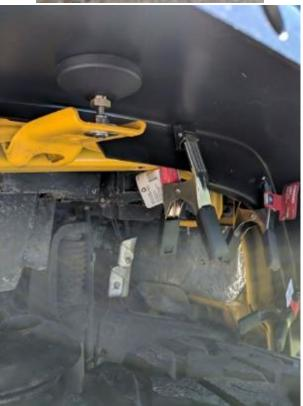
8. Once the fender is lined up, put [2] 1" button head bolts with the larger washers through the front two holes that line up. Use the smaller washers on the back of the bolts with the locking nuts. Use the 5/32" allen wrench and the 7/16" end wrench to secure the two holts in place.
