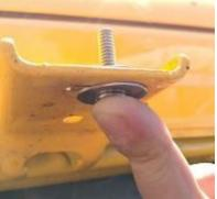
7. With the help of another person or clamps, hold the fender in its proper place to fit in the stamped body panel. You will notice the first two holes are the only two that line up with the factory holes on the Jeep.
