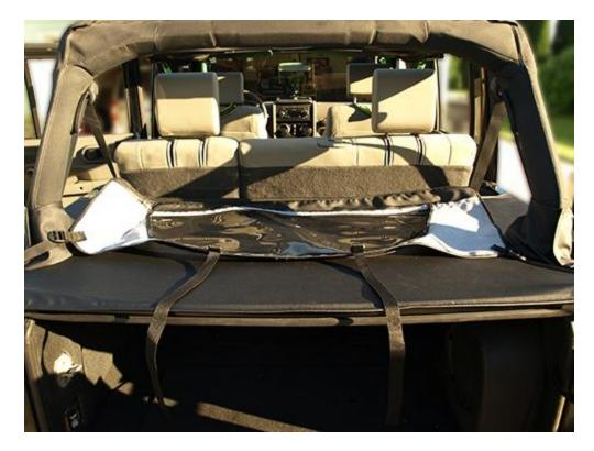
3. Drop down both rear passenger seats to easily access the MasterTop Zip Down Wind Stopper and MasterTop Tonneau Cover zippers.
