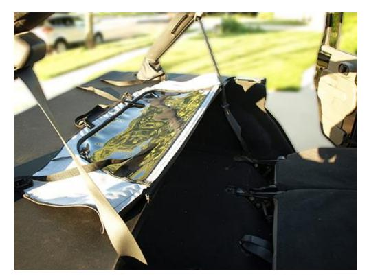
6. Wrap the two center straps of the MasterTop Zip Down Wind Stopper around the upper sports bar and secure the straps in the buckle. Do Not tighten the center straps just yet.
