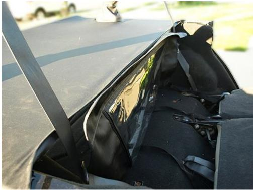
5. Flip the MasterTop Zip Down Wind Stopper up so that it lays on top of the MasterTop Tonneau Cover.
