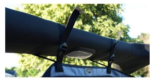
7. Wrap each side strap around the outer part of the sports part above the seat belt mounts and secure to the buckle of the MasterTop Zip Down Wind Stopper. Tighten the side straps and the center straps now.
