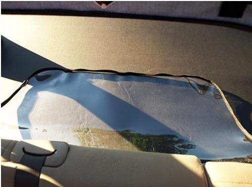
9. *Optional*: The open window of the MasterTop Zip Down Wind Stopper can be placed between the rear passenger seats and the MasterTop Tonneau Cover as shown below. Be careful not to damage the window when placing items in the trunk area.
