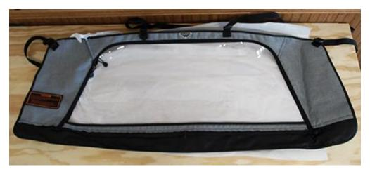
2. Lay the MasterTop Zip Down Wind Stopper with the zipper facing the rear passenger seats with the gray side up on the MasterTop Tonneau Cover.
