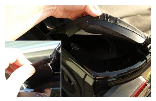
8. Secure the plastic strip along the side of the MasterTop Tonneau Cover into the side rail retainer channel. *Note:* Make sure that the plastic strip is all the way into the channel before sliding the opposite side into place. It may be tight when sliding the opposite side into the rail retainer channel.
