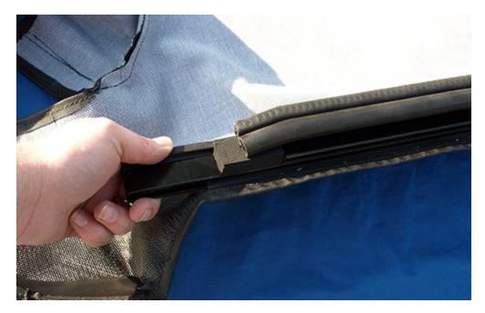
4. Place the MasterTop Tonneau Cover on the back of your Jeep®. Locking the ends of the tailgate bar into the side clamps.
