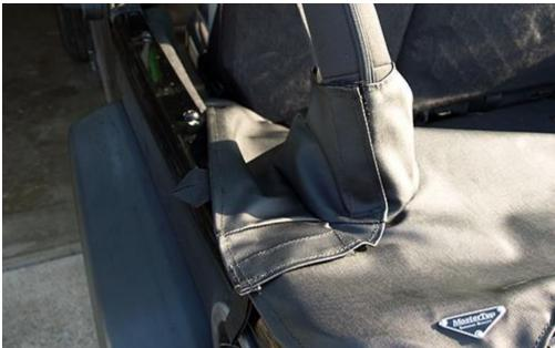
7. Secure the rear corners of the MasterTop Tonneau Cover. Place the plastic strip into the corner rail retainer channel.
