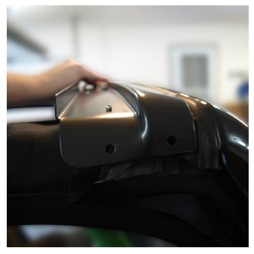
3. With the MasterTop Windshield Header in place you will take each Header Knob and place it through the hole of a Header Knob Plate with the angled end facing the Header Knob.
