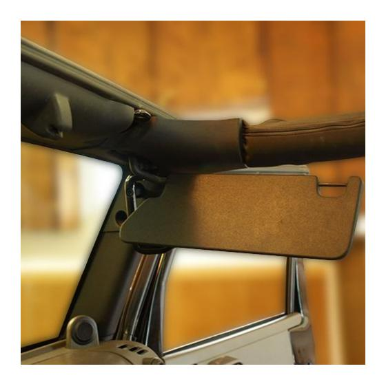
2. Once the sun visors are moved, place the MasterTop Windshield Header just behind the windshield and over the weather stripping. Each Knob Base should be right over the top of a footman loop.
