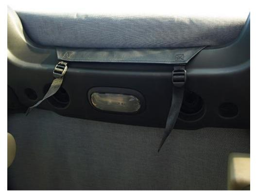
8. Secure the large hook and loop straps around the horizontal sports bar on the driver and passenger sides.
