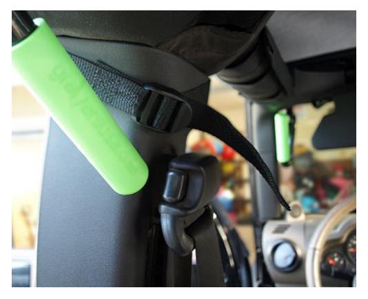
**Important Note:** Do Not thread tension strap under the seat belt. It should be above it as shown.
