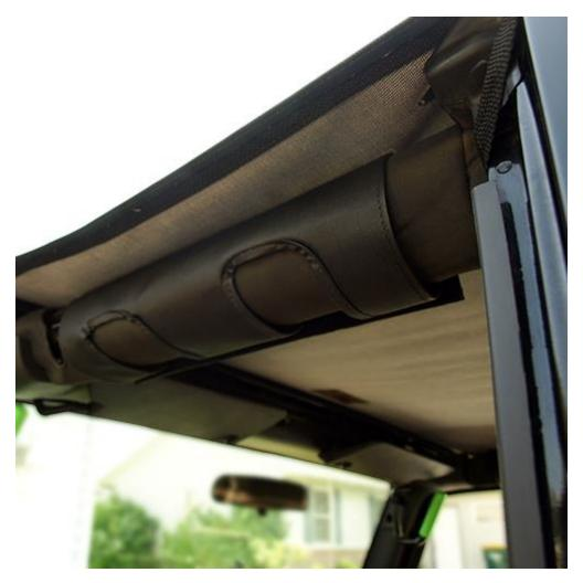
9. Place the exterior side tension straps around the driver side doorframe and thread the one end into the buckle. Repeat steps on both sides. Important Note: Do Not thread tension strap under the seat belt. It should be above it as shown below.
