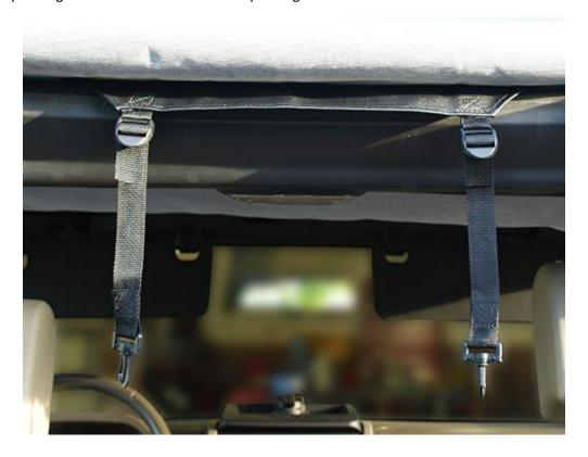
7. Secure each tension strap hook to the hole of the sports bar as shown below. With the hook in place, tighten the strap. Don't over tighten as you may break the plastic hook.
