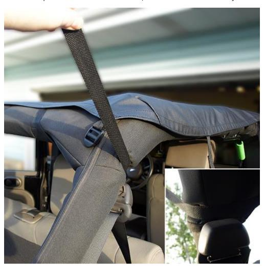
14. With a twist of the tension strap, so that it lays flat on the sports bar, thread it through the buckle and pull tight. The buckle should lay flat against the sports bar. Repeat steps on opposite side.
