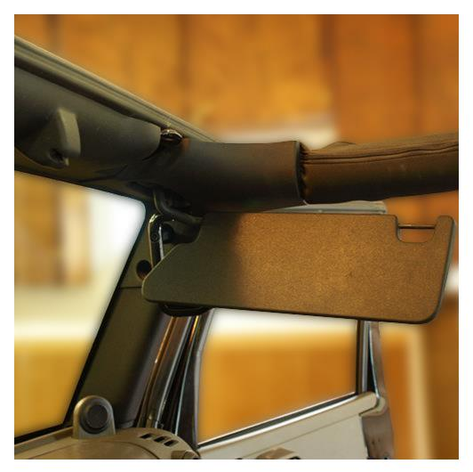
3. Now place the MasterTop Bimini Top Plus with the gray side facing down and secure the windshield header to the footman loops on the driver and passenger side.
