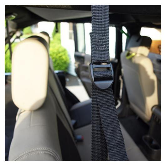
11. Place the large plastic hook under the lip right behind the rear passenger side door. Once in place pull up until the hook locks into place. With the hook secured, tighten the tension strap. Repeat step on opposite side.
