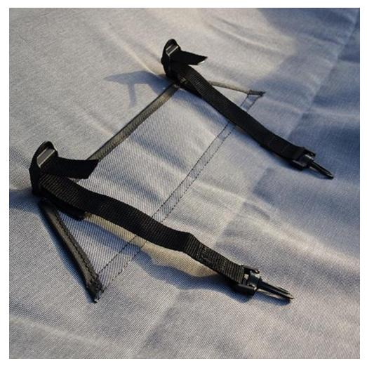
6. Once both tension straps with hooks are secured to the buckles, unfold the MasterTop Bimini Top Plus towards the rear passenger seats. Let the tension straps hang down.
