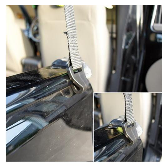
**Note:** If you have a hard top there may be a rubber gasket that is towards the rear passenger side door. As shown in the picture above, you will need to place the hook just to the side of the gasket and then pull it up into the lip.
