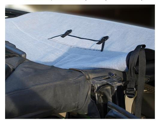
5. Thread the short tension straps with hooks through the buckles on both sides of the MasterTop Bimini Top Plus.
