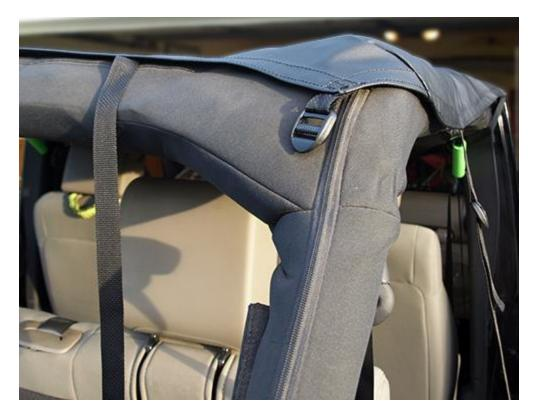
13. The rear tension strap will need to be pulled under the rear sports bar and to the exterior. **Important Note:** *If* placing the tension strap under the rear seat belt mount, make sure it DOES NOT interfere with the seat belt.
