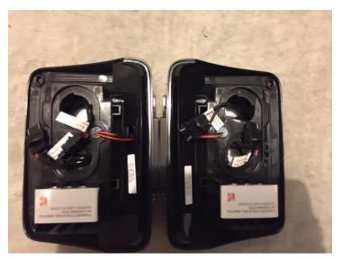
5) Take the old wiring harness and connect it to the corresponding wires on your new taillights.
