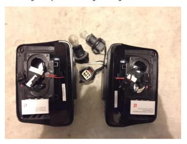
4) Locate the 2 plugs which are pushed inside of your new taillights and pull them out. Be careful not to touch any of the circuitry on the lights while doing so to avoid static discharge.
