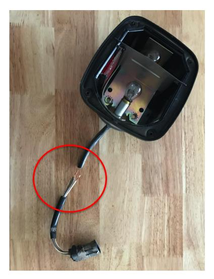
Step 8 – At this time you must determine which wires perform what function on the vehicle. With the Jeep in Park and with the emergency brake applied, turn the ignition to the "On" position. Do not start the vehicle at this time.
