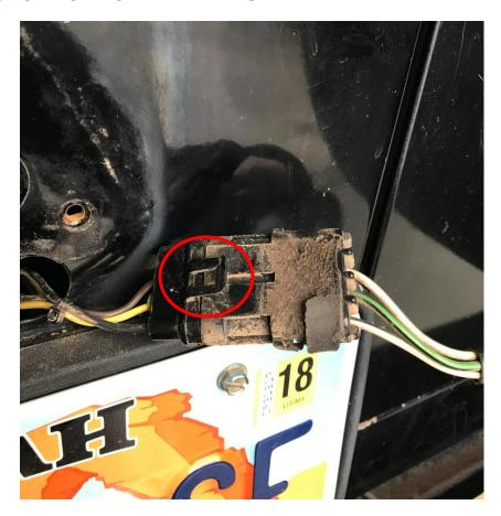
Step 5 - Next, cut the existing harness about halfway between the connector and the taillight. The existing harness will be attached to the new light.
