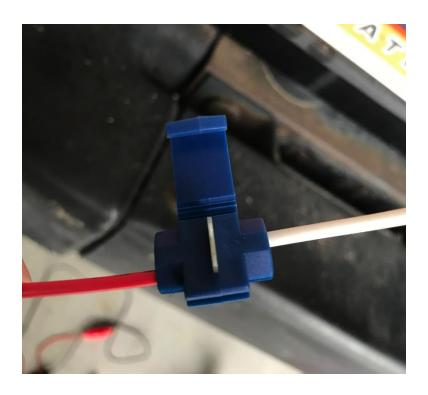
Step 15 - Fold the center of the splice block over until it clicks and snaps into place.
