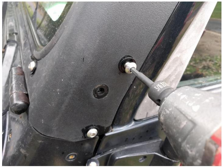
5. Loosely install base bracket in location on pillar. Brackets will be tightened at completion of installation. Note: On TJ installation, passenger-side base bracket DOES contact stock antenna resulting in an annoying rattle while driving. Might be a good time to replace antenna with a rubber stubby.
