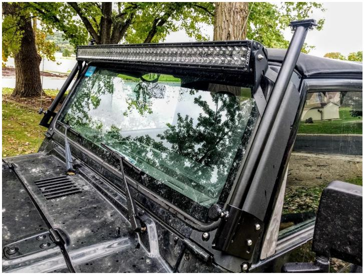
7. Lay crossbar across top of Jeep and carefully thread T-slot in crossbar onto first upright post. Moving to opposite side, slide crossbar far enough onto first post to thread onto second post. Center crossbar for even spacing. Hand-tighten knurled bolts on bases.
