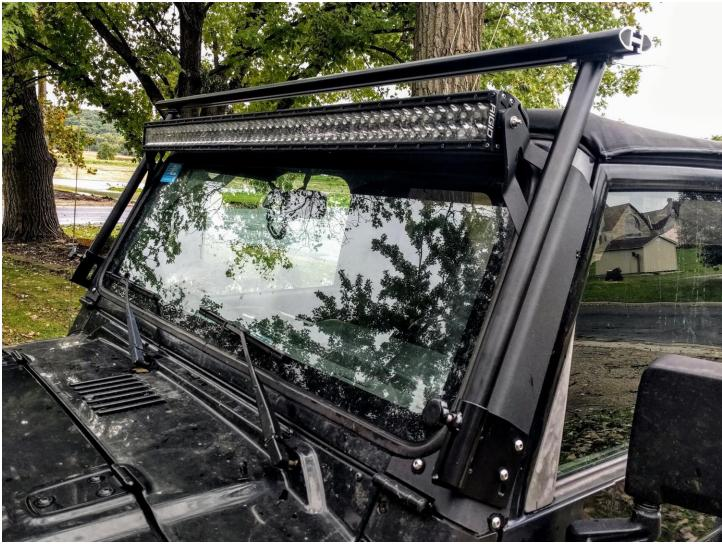
8. Install End Caps and tighten 1/4in upright post bolts with 7/16 wrench or socket. Go back and securely tighten bolts on base brackets.
