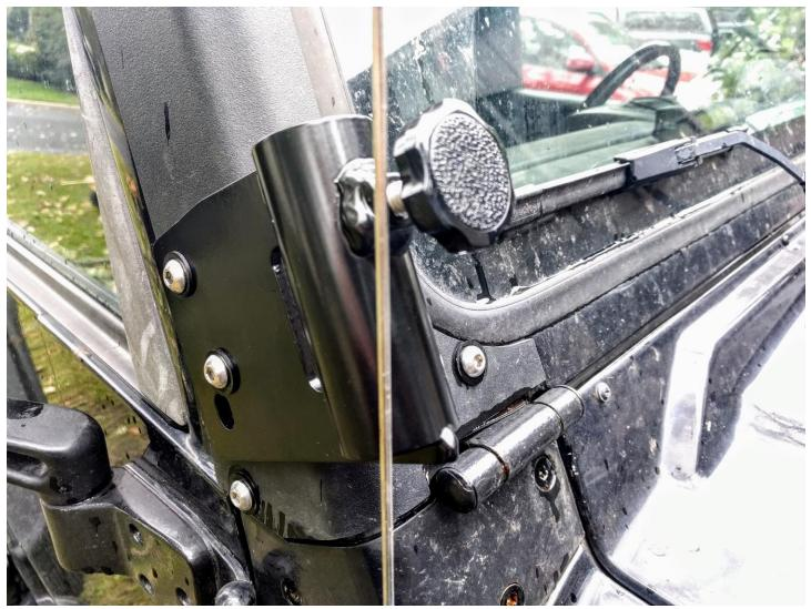
6. Identify RIGHT and LEFT uprights (They are not marked. Drop one into place and verify whether top crossbar mounting point is level. If not, switch them and check again.) Insert into bases but do not tighten.
