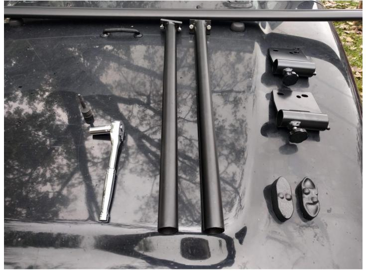
2. Prestage 1/4 in bolts in the top brackets of upright posts. Powder coating on inside of bracket threads may make bolt insertion difficult, be careful not to crossthread.
