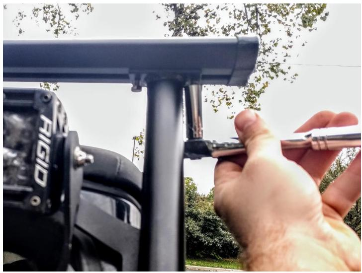
9. Final Note: If crossbars sit higher than necessary above vehicle, upright posts can be cut at bottom to lower overall height. Alternatively, base brackets allow some flexibility to raise assembly as desired.
