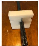
4. Now assemble the remaining larger form pieces with the fingers oriented upwards and the smaller slot on the left hand side like the previous foam piece. Be sure to leave the assembled foam piece behind the tab with multiple mounting holes to ensure it does not interfere with cable operation.
