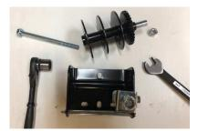
3. Mount the crank assembly using the (2) supplied 3" lag screws and washers. Once mounted reinsert the spool and attach the supplied handle as shown.
