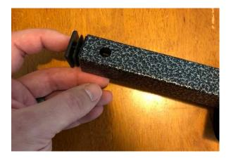
7. Attach elastic straps to the grommets then to the main frame for now. These will be used later to secure the Freedom Panels to the frame prior to lifting off the top.
