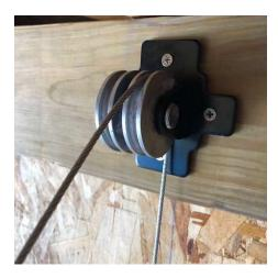
6. Loop the cable through the front mounting tab on the assembled frame and tighten using the supplied hardware as shown.
