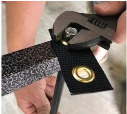
6. Attach the rear hook assembly as shown using the supplied nylon nut. Be sure not to overtighten as adjustment will be necessary during hard top removal. Insert square plugs into the exposed ends of the tubes.
