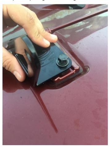
4. Tighten the nuts with a 1/2" socket until it is tight, but do not overtighten.
