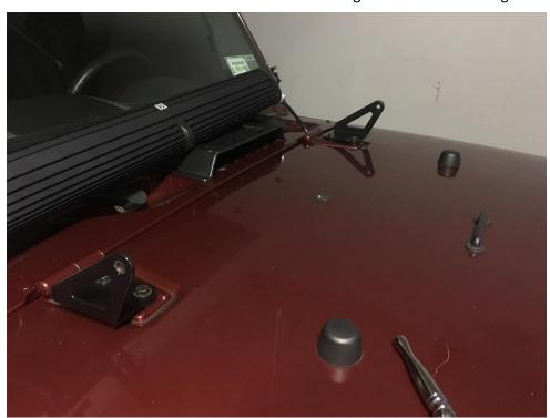
7. You can now insert the KC HiLiTES 30 in. C-Series C30 LED Light Bar to the Hood Mounting Brackets using the screws included with the light bar.
