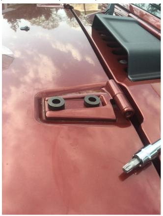
3. Align the holes on the KC HiLiTES mounting bracket with the spacers and place the washer and nut as shown. NOTE: This is the correct setup for the passenger side mounting bracket.
