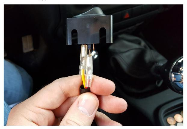
14. Attach one end of the BROWN ground wire to the switch terminal marked EARTH.
