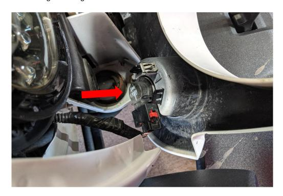
5. After turn signals are removed pull the rest of the grille off the vehicle. There will be a few retaining clips at the bottom of the grille.
