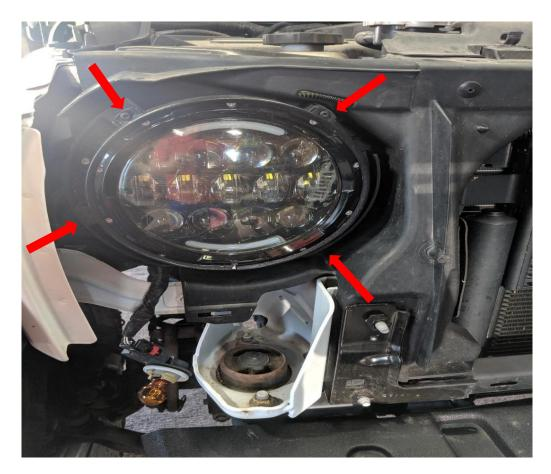
7. Using your T15 torx driver, remove all 4 screws per headlight.
