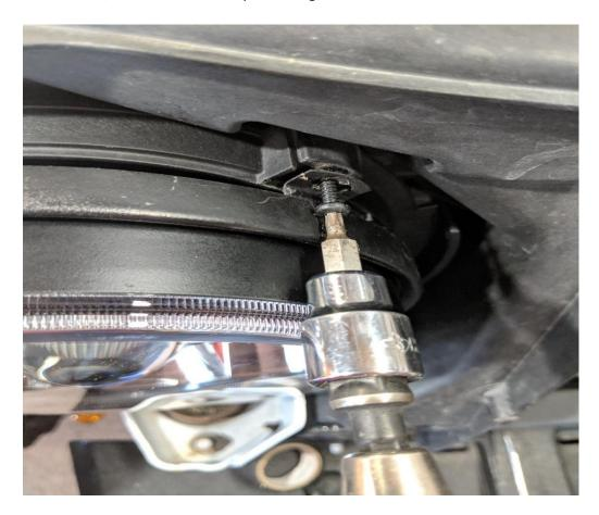
8. After the retaining ring is removed pull out the existing headlight and remove the headlight from the H13 connector.
