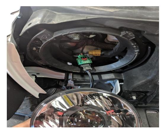
11. Now put the new headlight into place and secure with the retaining ring and retaining screws.
