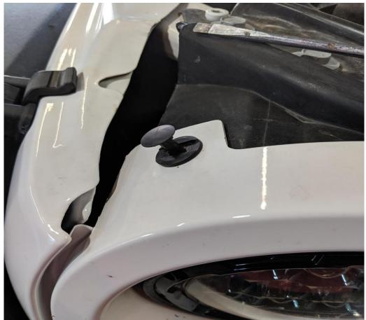
3. After all the clips are removed carefully pull the grille out towards you.
