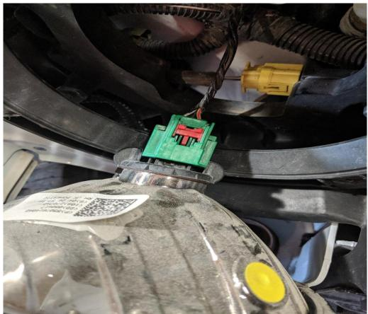
9. Apply some dielectric grease in the connector that was provided with the new headlights.
