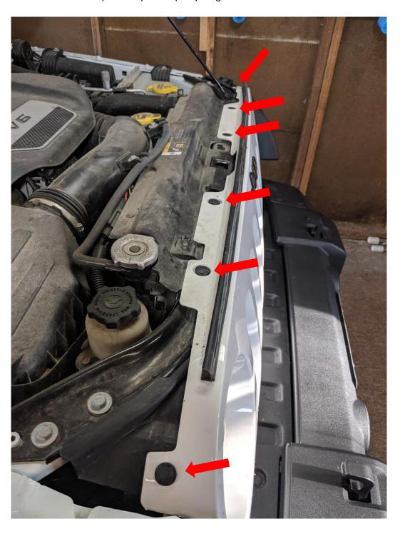
2. Take your flat-head screwdriver and carefully pry up the center pin on all 6 plastic clips.
