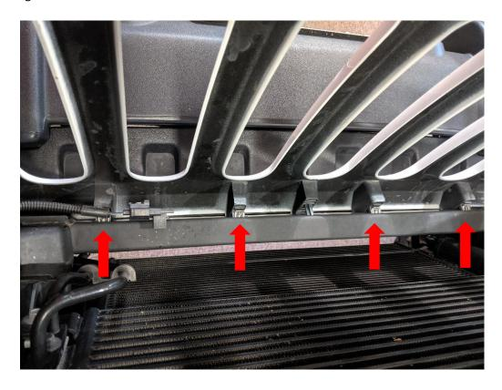
6. Now locate the retaining ring and retaining ring screws around the headlights. There are 4 screws per head light.
