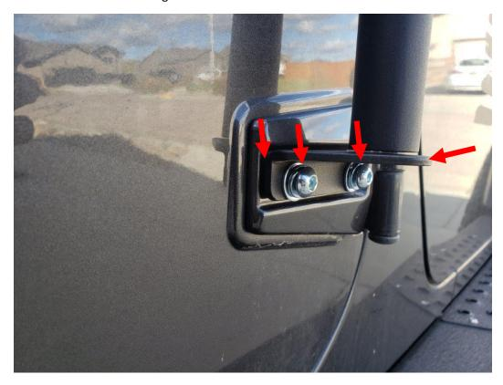
**6.** Install the lower bracket bolt, washer, and lock washer as shown. Fully tighten using a 5mm hex. Then fully tighten the bottom 2 hinge bolts using the 5mm hex.
