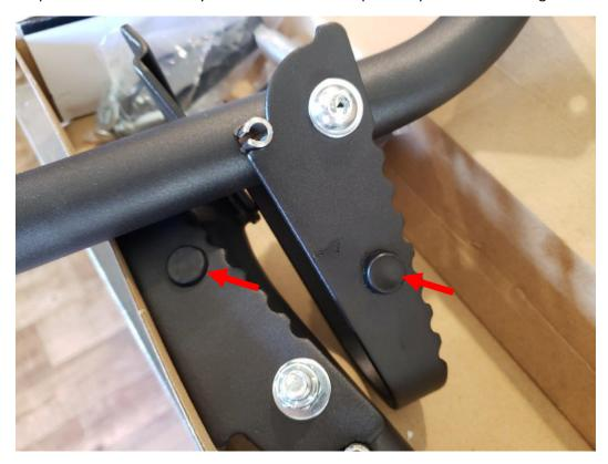
2. Using a T50 torx bit, remove the 2 bolts from ONLY the top hinge. It is important to leave the bottom hinge bolts fully tight at this point.
