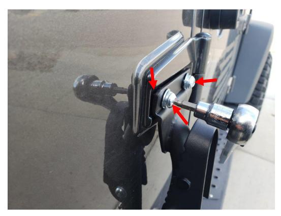
**4.** Next, use a T50 torx to remove the 2 lower hinge bolts.
