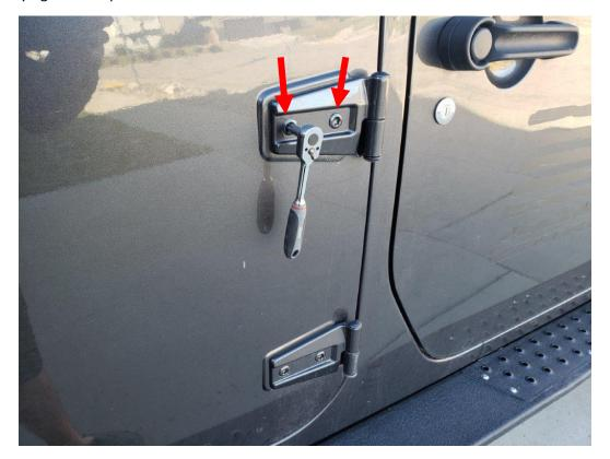
**3.** Using the supplied bolts, washers, and lock washers install the upper step assembly as shown. Be sure to use the supplied rubber gasket between the bracket and the door hinge. Using a 5mm hex bit, fully tighten both bolts.
