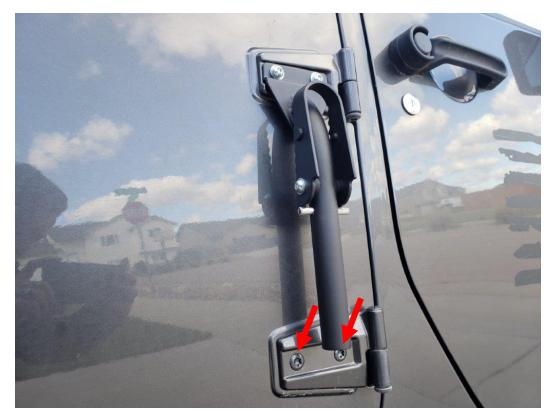
**5.** Then install the lower bracket as shown. Place the rubber gasket, then the bracket, then insert the bolts with washers and lock washers. Just snug them for now.
