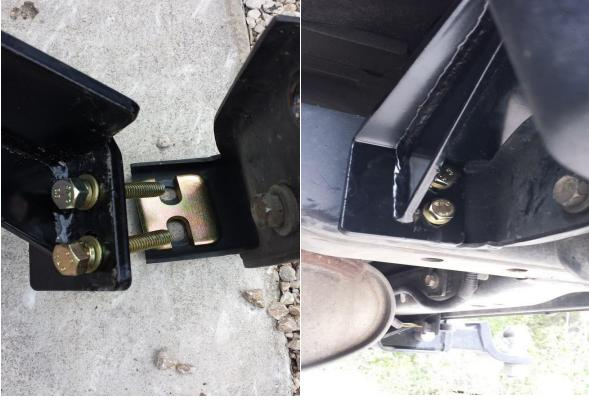
5. Install the 'U' bracket onto the carriage bolts with the 5/16" nyloc nuts, washers and 1/2" socket.
