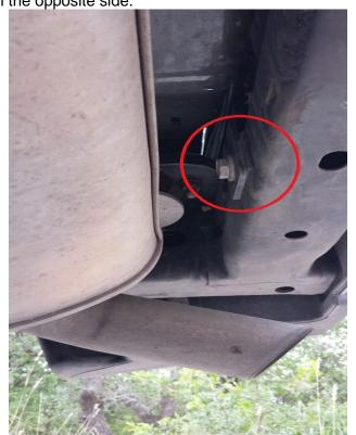
4. Slide the rack support mount between the bumper and the body, insert 2 supplied carriage bolts. Place the provided 'H' spacer in the stock bumper mount and the new mount and install the provided bolts, lock washers and washers with a 5/8" socket. Reinstall the stock bumper bolt in the rear of the frame, (removed in step 3). Do the same on the opposite side.
