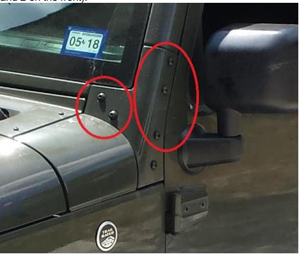
2. Install front hoop with the 10, M8x35mm bolts, lock washers, washers and nylon spacers provided, with a 6mm Allen wrench.
