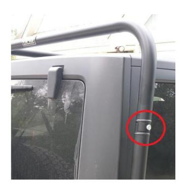
9. Place the roof rails on top of the Jeep with the straight end towards the back and the bent end towards the front. Install the end caps with 6, 5/16" socket head cap bolts and 1/4" Allen wrench.
