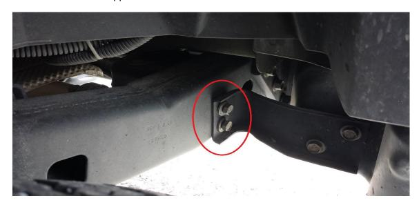
Remove the stock bumper bolt in the rear of the frame with a 5/8" socket. (This will allow the rack support to slide in easier between the bumper and body). Do the same on the opposite side.
