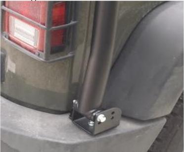
8. Attach rear upper hoop to the rear uprights with a 1/2" socket head cap screw, 1/2" nyloc nut and a 3/8" Allen wrench.
