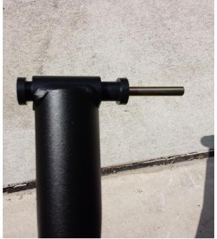
7. Install the rear upright, bushing end into the 'U' bracket and install 3/8" Hex bolt, lock washer and washer with 9/16" socket.
