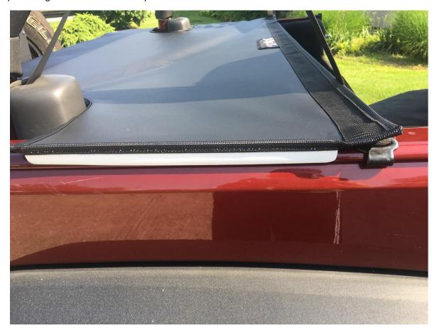
6. Take the metal hook attached to the bungee strap and slide it under the lip
