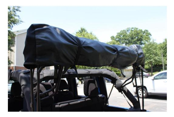
14. Finish tucking in the fabric, pull the straps tight and engage the locks.
