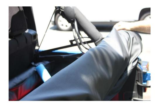
6. Slide the boot over the folded top starting at either side and working across.
