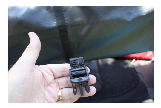
10. Reach under the boot and fasten the center strap. Leave it unlocked and loose at this time.
