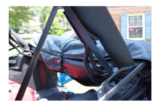
12. Now tighten the three straps tucking the front flap in as you go. Leave the buckles unlocked.
