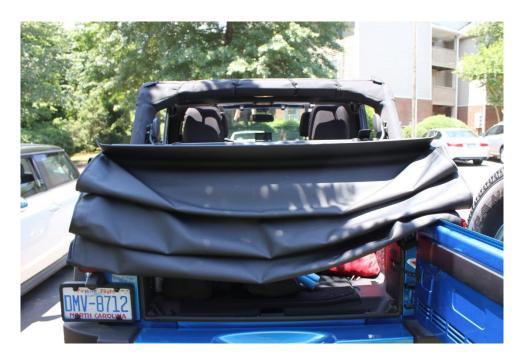
5. Grab the fabric from the bottom and fold up over the front frame. Fold the latches in the closed position so they don't poke the top fabric.
