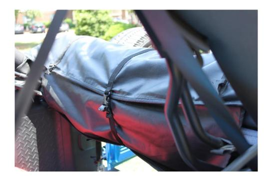
11. Tucking the front flap in at the bottom as you work across, fasten the other two straps.
