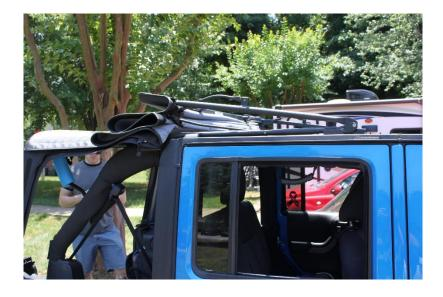
3. Open the tailgate and release the rear corners. Lower the top, again pulling the fabric away from the bows.
