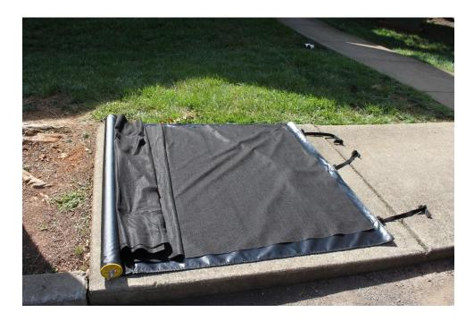
9. Place rear window with bottom toward tube and inside facing up. Make sure window plastic is on fabric.
