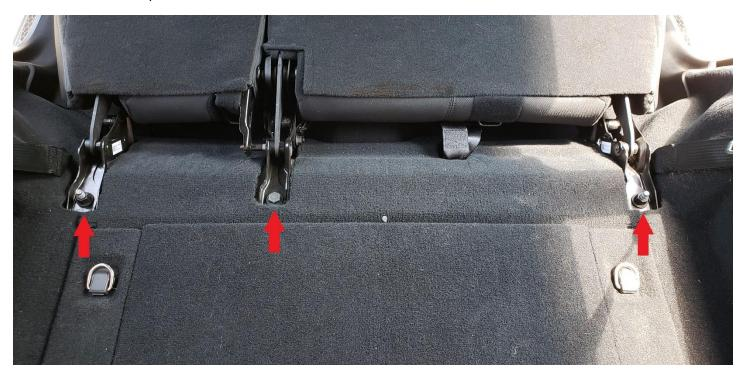
2. Using the same 18mm Socket, remove the 4 bolts securing the 4 seat legs to the floor. (These 4 bolts will be replaced by those included in the kit)
