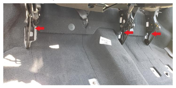
5. Now place 1 square spacer under each of the 3 seat brackets, lift the bracket and slide the spacer in. Insert the factory bolts and tighten, ensure the spacer is square to the seat bracket and not twisted. Tighten to manufacturer specifications (45ft/lbs).
