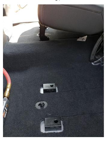
7. Insert the new SEM Bolts and hand tighten, ensuring the spacers continue to stay square with the seat legs. Tighten all 4 SEM Bolts to manufacturer specifications (45ft/lbs).
