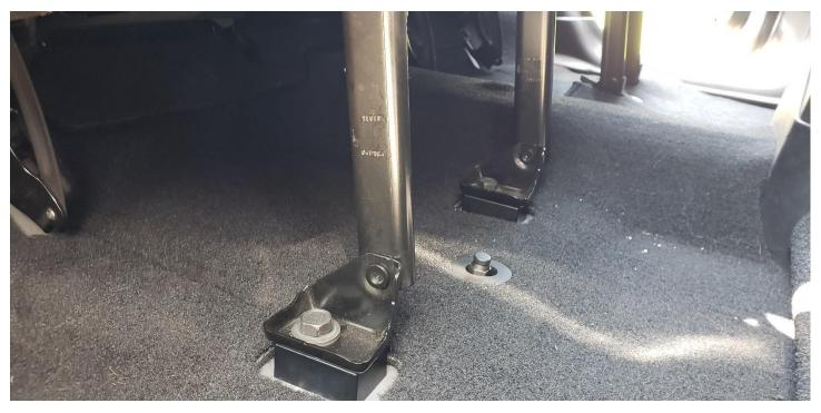
8. Re-tighten the 3 fasteners behind the rear seat to manufacturer specifications (1 bolt - 45ft/lbs) (2 nuts – 62.5ft/lbs).
