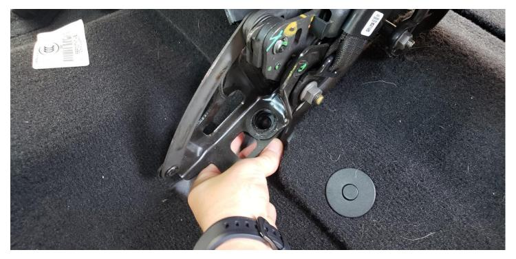
6. Place 1 rectangular spacer under each of the 4 seat legs, with the hole towards the rear of the Jeep.
