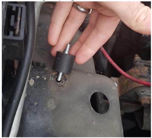
6. Use 10mm nut and washer from underside of the passenger fender to secure vibra-mount.
