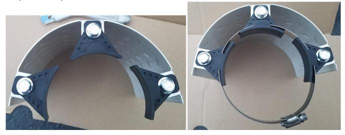
14. Place filter into hose clamp on the heat shield. Adjust hose clamp to be centered on filter neck.
