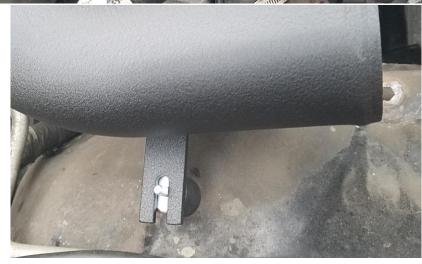
**Note:** A 1 Inch motor mount lift required the throttle body side of the intake tube to be shortened for proper fit. This may not be required for stock motor mounts.
