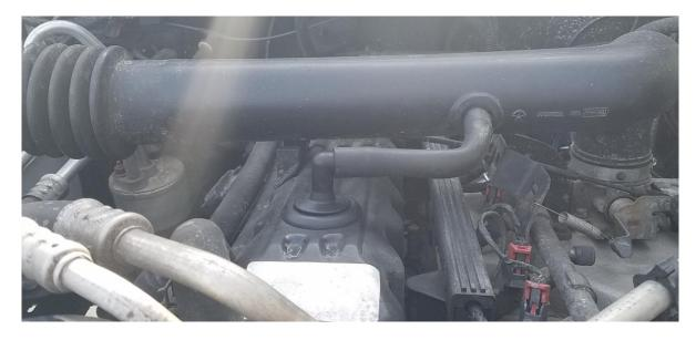
4. Remove stock intake tube from throttle body.
