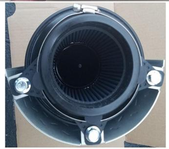
15. Place filter neck over intake tube. Make sure the filter slides completely over the intake tube lip and adjust so heat shield is facing the engine. Check for proper alignment and free of moving parts. Once properly adjusted, tight 8 mm bolt on hose clamp and 1/2 Inch heat shield bolts. Do not over tighten all bolts or clamps.
