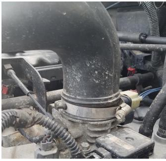
2. Remove air box top and filter. Remove thee 8 mm bolts connecting air box to the passenger fender. There is an 8 mm nut on the inside of the fender for each bolt.
