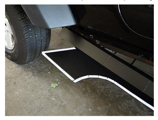
3. Remove the tape liner from the automotive double-sided tape.
