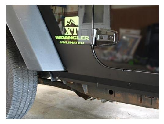
6. Bend the bottom finger tabs up around the pinch seam. These tabs will help hold the rocker guard in place.
