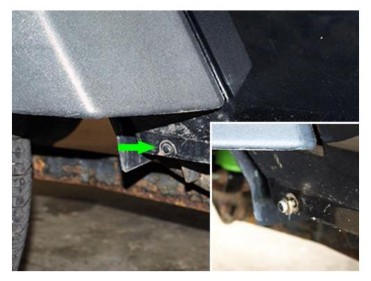
2. Clean the entire area where the rocker guard will be placed with soap and water or another cleaning solution. Clean the area where the automotive double-sided tape will attach to the Jeep® with rubbing alcohol.
