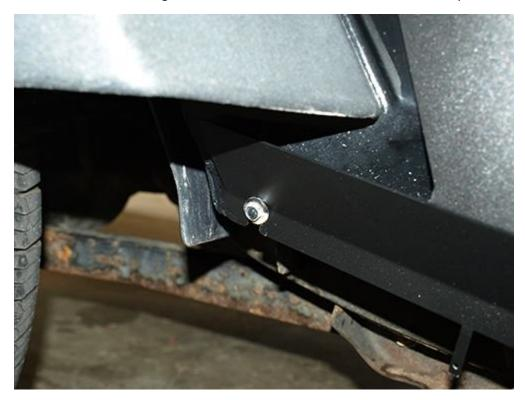
5. Align the rocker guard with the edge just under the door well. *NOTE:* The automotive double-sided tape is very strong and will not remove easily once placed on the Jeep®. Take your time positioning the rocker guard. Push firmly against the rocker guard where the tape is secured to the Jeep®.
