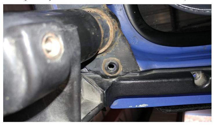
7. Install the handle with the 2 T40 factory screws.
