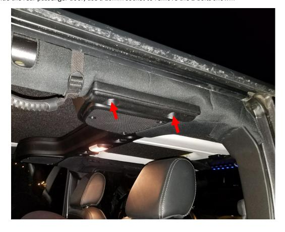
**8.** Using the supplied bolts and 5mm hex wrench, install the rear handle as shown below. The handle should be facing forward. Torque both bolts to 120 in/lbs.
