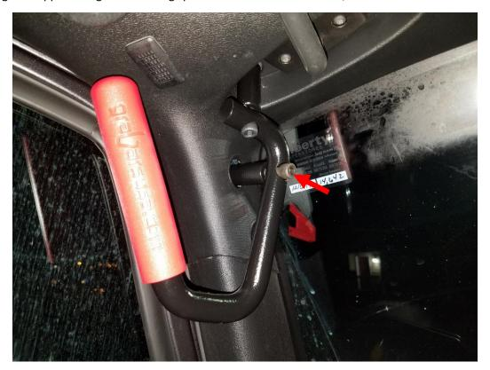
5. Using a 6mm hex wrench tighten both the upper and lower bolts. Toque both to 300 in/lbs.
