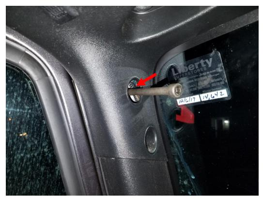
**3.** Using the supplied short bolt and short spacer with a 6mm hex wrench, install the handle as shown. Only thread the bolt a few turns for now. *Note: The front handles are driver/passenger side specific. The correct handle should tilt toward the window as shown below.*
