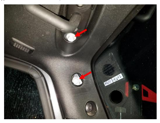
2. Using one of the long supplied bolts, hand tighten it into both of the bolt holes from step 1. There is usually a buildup of loctite that makes this bolt want to cross thread. Thread this bolt in and out of the holes to clear out the threads. This will make install much easier in the next steps..
