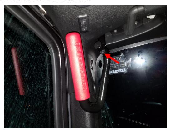
**4.** Using the supplied long bolt and long spacer with a 6mm hex wrench, thread in the lower bolt shown.
