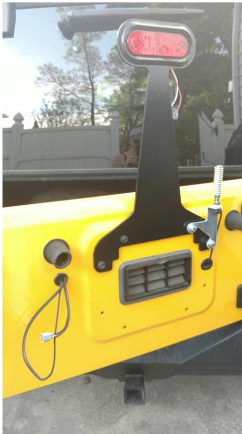
4. Use wire cutters to cut the stock wire harness close to the plug.
