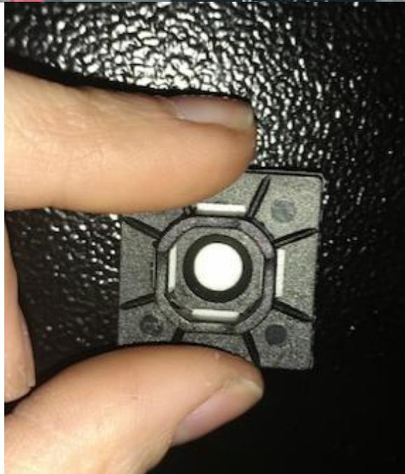
13. Remove the adhesive backing of each mount and place them on the bracket. Thread a zip tie through each mount to secure the wires in place.
