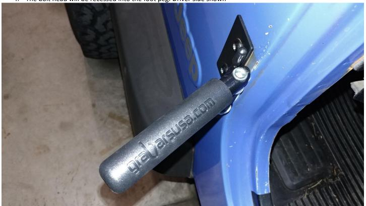
5. Insert the bolt then one washer, insert the bolt into the hinge finish off with one washer and then the nut.
