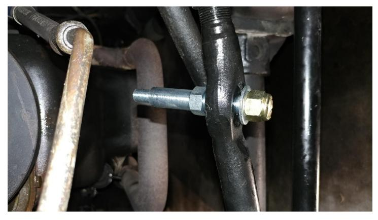
8. The new FOX 2.0 Performance Series IFP Steering Stabilizer will be hard to compress. To make installation easier I maxed out the steering to the driver side. This makes the distance between the drag link mount and frame mount almost equal to the steering stabilizer length.
