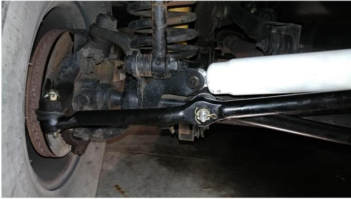
5. To access the bolt you may have to turn the wheel. To make the drag link and tie rod move.
