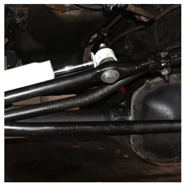
4. Remove the frame mount side of the factory steering stabilizer. Using a 15mm open end wrench and 18mm socket
