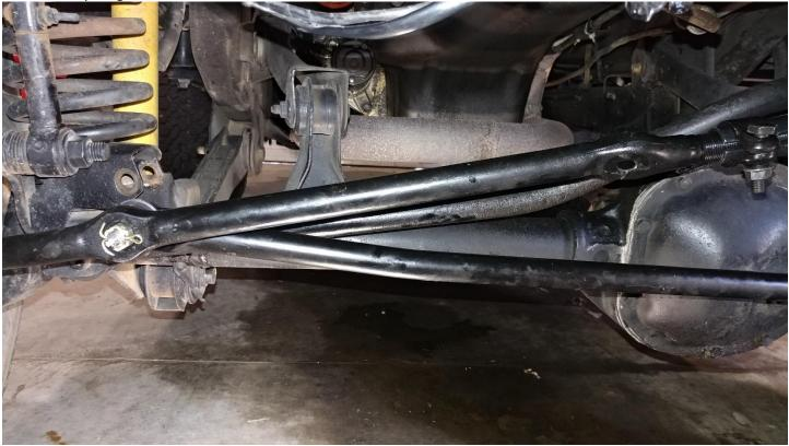
7. Using a 3/4" open end wrench and 3/4" socket press the tapered end of the new stud into the drag link location.
