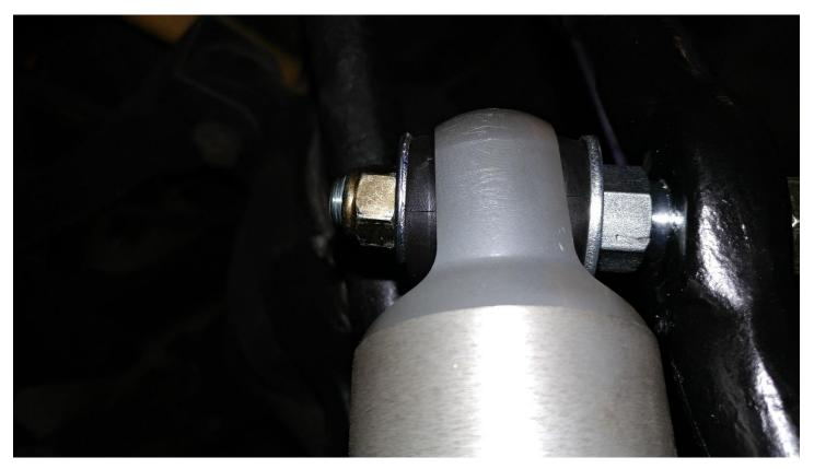
10. Reinstall the factory bolt and nut on the frame side. Using a 15mm open end wrench and 18mm socket.
