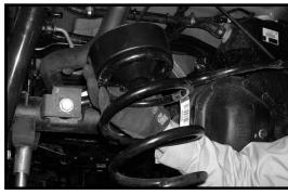
21. Working on the driver side, carefully push the stock ABS clip back into the bottom side of the stock frame rail. Repeat procedure on the passenger side. Special note: Take care not to damage the stock ABS clip during installation.
