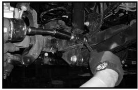
9. Locate the stock front end link mounting hardware. Working on the driver side, install the stock front sway bar end link into the stock lower mounting location and secure using the stock hardware. Make sure to use thread locker or loctite and torque to **45 ft lbs.** Repeat procedure on the passenger side.
