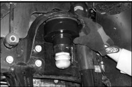
7. Locate the stock driver and passenger side coil springs that were removed in step # 4. Working on the driver side, install the driver side coil spring into the stock location. Repeat procedure on the passenger side. Carefully raise
