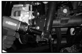
stock coil spring. Now install the stock isolator on top of the on the driver side, install the stock rear sway bar end link into new rear coil spring spacer and install the stock coil spring, the stock lower mounting location and secure using the stock new rear coil spring spacer and stock isolators back into the|hardware. Make sure to use thread locker or loctite and
