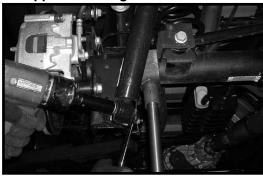
16. Working on the driver side, remove the lower mounting hardware that connects the stock sway bar end link to the stock lower bracket that is attached to the rear axle. Save the stock hardware for later re-installation. Repeat procedure on the passenger side. Let the stock sway bar hang.
