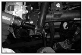
24. Locate the stock end link mounting hardware. Working on the driver side, install the stock rear sway bar end link into the stock lower mounting location and secure using the stock hardware. Make sure to use thread locker or loctite and torque to 45 ft lbs. Repeat procedure on the passenger side
