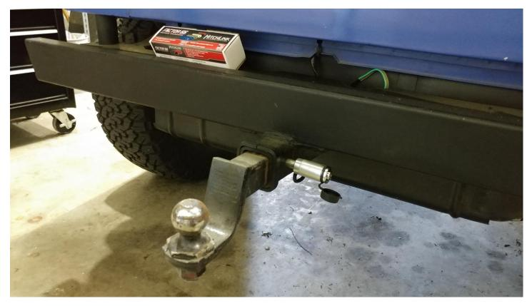
2. If using a locking receiver pin, unlock the pin
