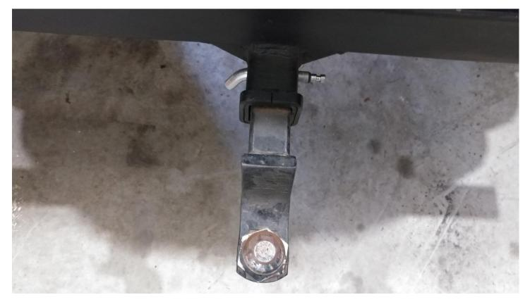
3. Remove the receiver pin
