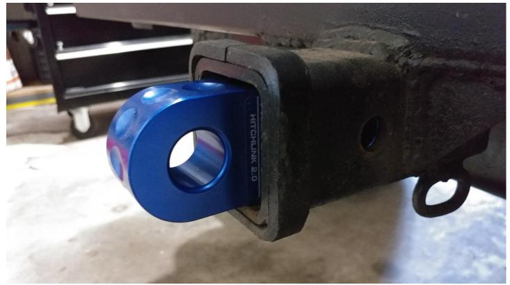
7. When the desired hole is found install the receiver pin
