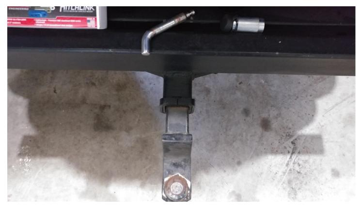
4. Remove the existing hitch in the receiver
