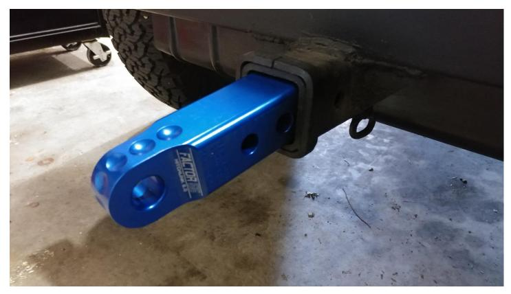
6. The Factor 55 Aluminum HitchLink 2.0 has two mounting holes the receiver pin can be used in
