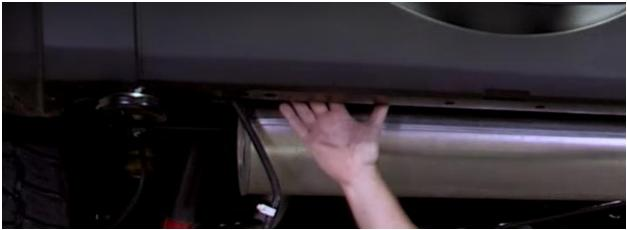
3. Start by loosening both bolts one full rotation; just enough to get the bolts to start turning a little easier. Now fully remove the TOP bolt. Then, fully remove the bottom bolt. Remove the tab. Complete this step on both the passenger and driver side of the vehicle.
