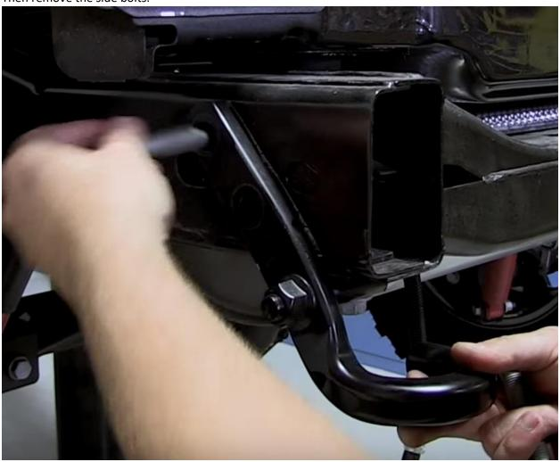
8. Fully remove the bottom bolt and then slide the entire bracket out.
