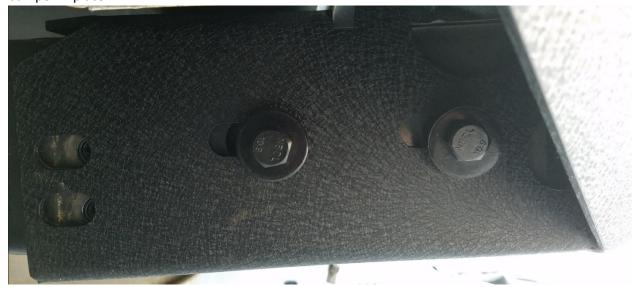
7. Once both sides are finger tight, work on fitting the bumper correctly to the body so that it is even on both sides of the Jeep. BE CAREFUL NOT TO SCRATCH YOUR PAINT WHILE MOVING THE BUMPER. Try to keep approximately 4mm of spacing under your rear fender. This will help avoid any rubbing when the vehicle flexes going over obstacles. It may be necessary to add a small piece of soft sided adhesive Velcro between the bumper and the fender if the fit on your vehicle is too tight.
