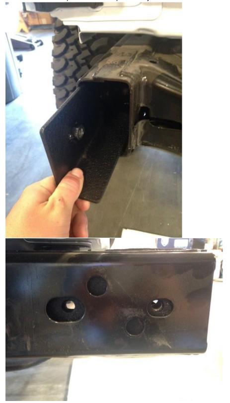
5. Using a friend, lift the bumper into place and rest it on the frame rails underneath the Jeep.
