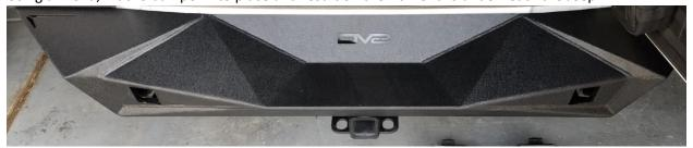
6. On each side, take two of the included bolts, lock washers, and washers and loosely place the bolts through the openings and into the nut plates in the frame rail to temporarily hold the bumper in place.
