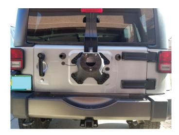
2. Remove the stock spare tire carrier by removing the 8 bolts using a 13mm socket or wrench.
