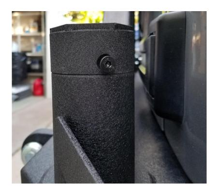
h. Install the hinge stop bracket on the bumper, to the right of the hinge, using the 2 13mm bolts with washers.
