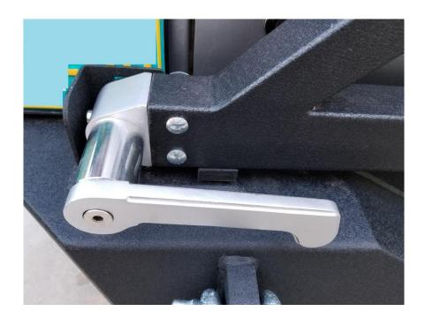
12. Using the 4 shorter 18mm bolts with washers, attach the tire adapter to the tire carrier, adjusting the height as needed for your tire size. Secure the bolts with the 19mm nylon nuts. This may require some trial and error as you should install it as low as possible.
