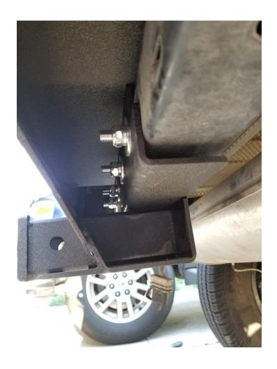
b. Install the 4 shorter bolts with washers, 2 on each side, into the nut plates installed in step 7 using a 19mm socket or wrench. Leave the bolts a bit loose for now.
