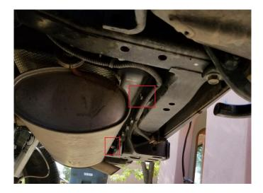
c. Rotate the 2 center brackets from a vertical position to a horizontal position so they don't hook onto the frame when removing the bumper, then pull the bumper out and off.
