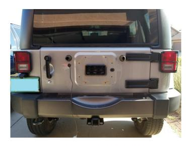
3. Remove the 3<sup>rd</sup> brake light from the stock tire carrier by removing the 4 screws using a size 20 Torx driver. Remount as desired. Alternately, wiring may be unplugged from the break light and stored inside the tailgate or rerouted as desired.
