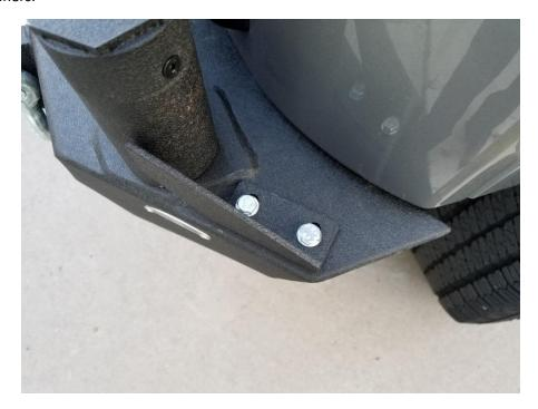
11. Install the tire carrier handle by sliding the rectangle end of the handle into the left hand end of the tire carrier and secure with appropriately sized bolts.
