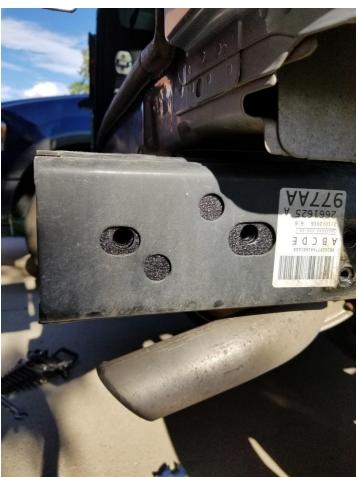
8. Insert the 4 large 4" 18mm bolts with washers through the rear frame rail from behind the rail, threads pointed toward the back of the Jeep. You will want to insert them by angling the head of the bolts above the muffler.
