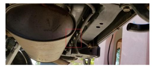
6. Remove the rear recovery tow hook (if equipped) by removing the 3 lighter colored bolts using an 18mm socket or wrench.
