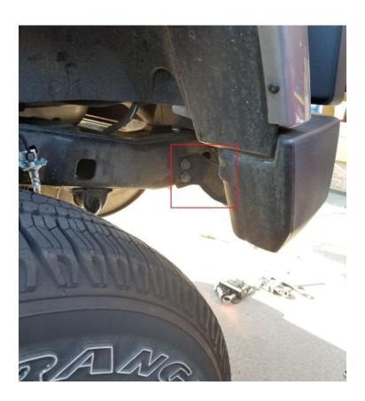
b. Remove the 2 lower bolts from the center brackets located about a foot from the center of the bumper on each side. This requires a 5/8" socket or wrench.
