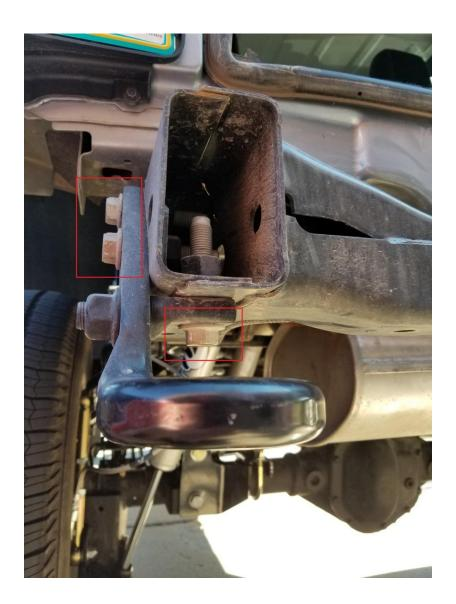
7. Insert the 2 nut plates into the frame rails, lining up the nuts to the factory holes in the frame.
