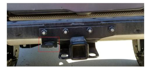
b. Remove the 4 bolts from the back side of the tow hitch using an 18mm wrench and slide the hitch off of the frame rail. You may opt to drop the muffler for easier access. Note that the nuts on the front side of the stock tow hitch are welded on.
