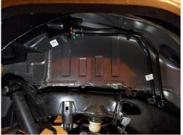
10. The new inner fender liner will leverage one of the mounting in the body of the vehicle. To enable this, the clip on the rear/lower portion of the fender will need to be removed. Use the trim removal tool and a plier detach the clip from the body of the vehicle.
