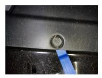
9. Now you can remove the inner fender liner. You might have to maneuver the inner fender out. If needed, use the trim removal tool to lose the inner fender liner from the clips in the outer edge of the factory installed fender.
