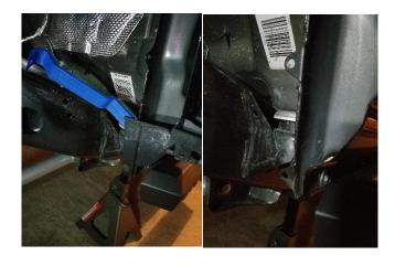
11. When working on the passenger's side, remove the grey plastic clip holding the line attached to the frame using the trim removal tool. The clip can be relocated (loosely) to the hole that is about one inch in front of original. This step won't apply when working on the driver's side.
