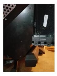
13. Using the provided hardware, the 3/8" socket and the 1/8" hex key, secure the bottom of rear portion of the inner fender to the two mounting holes in the body. You might have to maneuver the inner fender panel to ensure alignment with the mounting holes (Driver's side shown).
