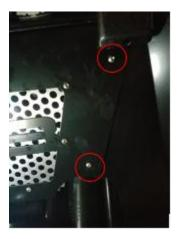
16. Using the provided hardware, the 3/8" wrench and the 1/8" hex key, secure the upper side of the front portion of the inner fender to the bracket on the fender (Driver's side shown).
