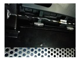
15. Using the provided hardware and the 3/8" socket, secure the front portion to the rear portion of the inner fender liner (Driver's side shown).
