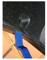
8. Release the inner fender liner from the 4 remaining clips in the rear of the fender. The clips should remain in place once the inner fender liner is detached.
