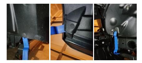
5. Using an 8mm socket, remove the 2 bolts in the front of the factory inner fender liner (Driver's side shown).
