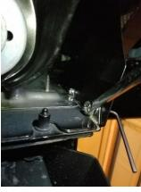
14. Now install the front portion of the inner fender liner. Make sure that the tab on upper portion of the panel gets inserted behind the body panel (Driver's side shown).
